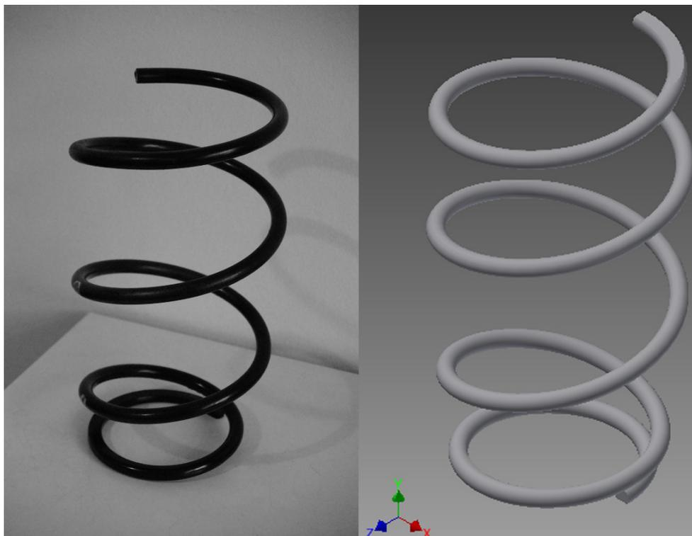
Fig. 3. Real (left) and modelled (right) spring geometry
