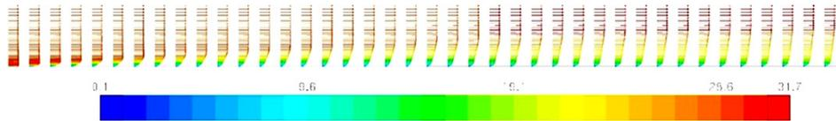
Fig. 9. The vector field distribution in the channel for the flow of  $e = 3.550$  and with a fixed velocity profile  $V_d$
