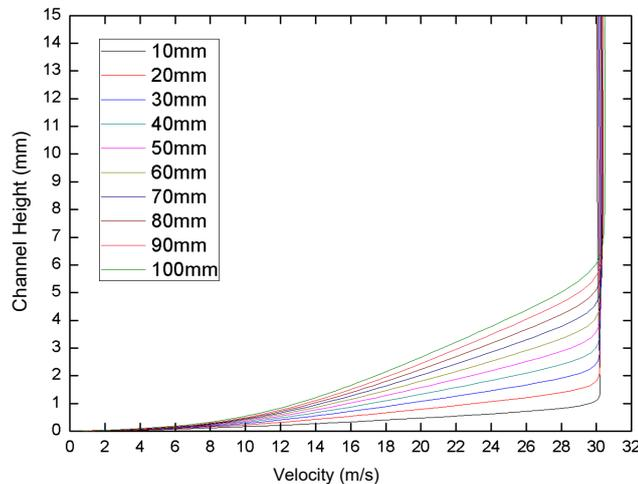
Fig. 5. Velocity distributions for each sections of channel for  $Re = 3,550$
