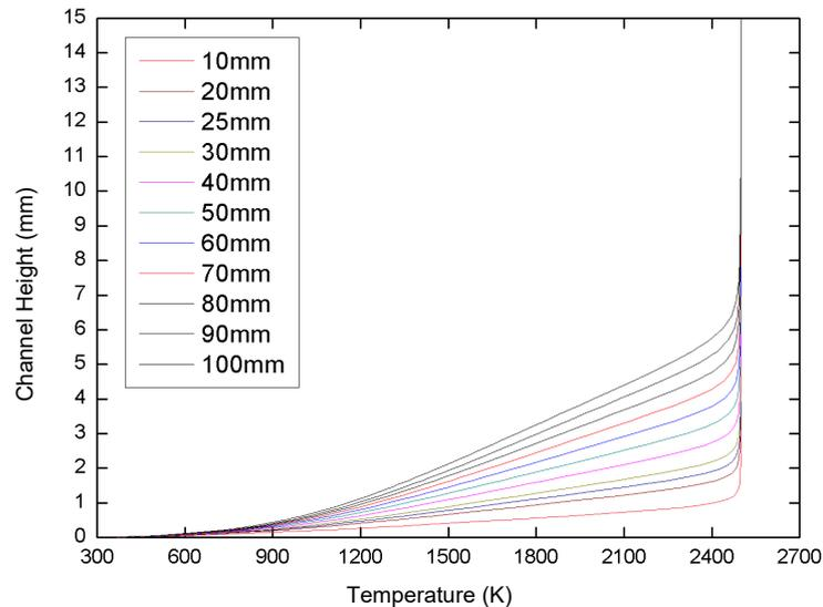
Fig. 13. Temperature distributions for each channel sections for the flow with  $R = 3,550$  and with a fixed velocity profile  $V_d$
