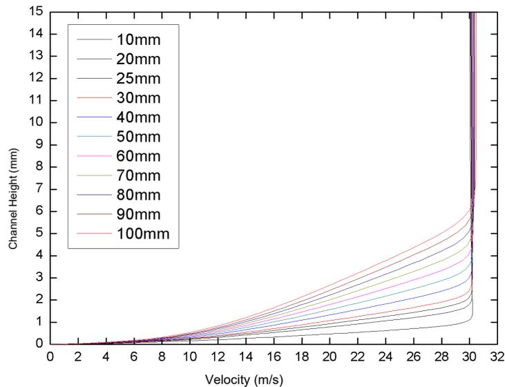
Fig. 12. Velocity distributions for each channel cross-sections for the flow with  $Re = 3,550$  for the velocity profile  $V_d$
