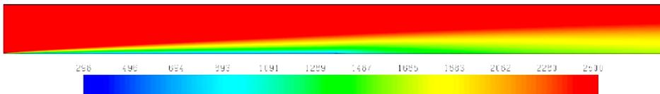
Fig. 11. The temperature distribution in the channel for the flow of  $Re = 3,550$  and with a fixed velocity profile  $V_d$
