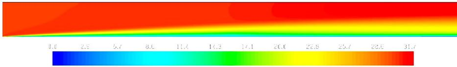
Fig. 8. Velocity field (modulus of two-component velocity) for the flow of  $Re = 3,550$ , and with a fixed velocity profile  $V_d$
