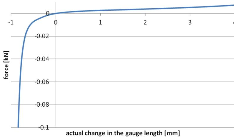
Fig. 4. Force versus actual change in the gauge length
