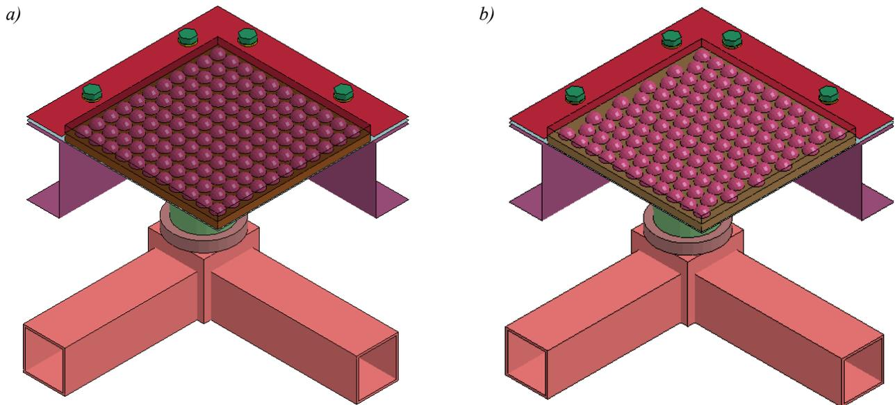
Fig. 3. An isometric view range stand with fixed panels for two variants a) parallel rows, b) moved rows
