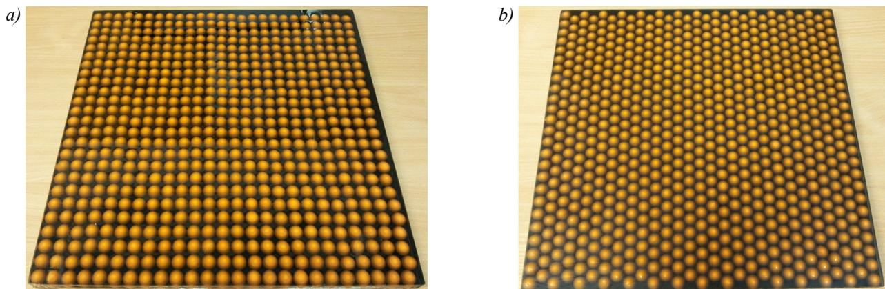
Fig. 2. Variants position liquid beads a) parallel rows, b) moved rows
