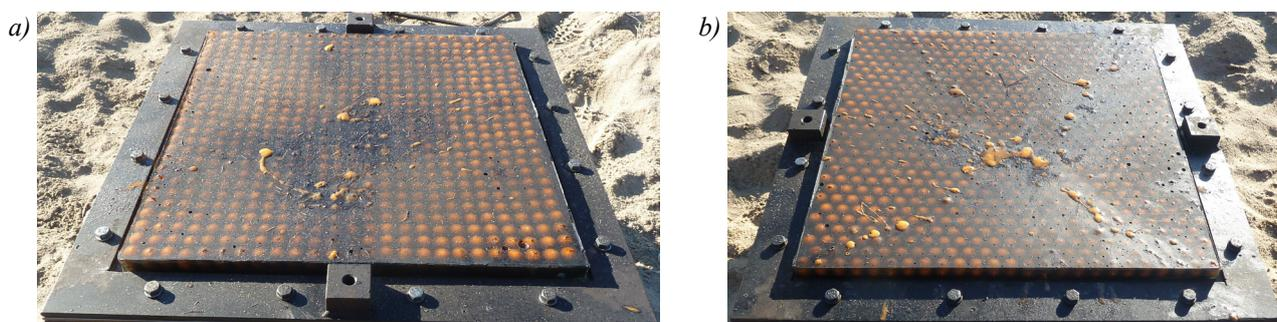
Fig. 6. The elastomer-liquid shield after 0.5 kg TNT blast test: a) parallel rows, b) moved rows
