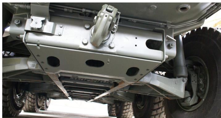
*Fig. 1. Integrated bottom frame for suspension and drive in ROSOMAK-type LAV vehicle*
