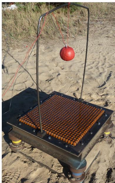
Fig. 5. The elastomer-liquid shield before 0.5 kg TNT blast test
