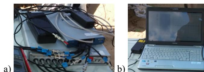
*Fig. 3. Fast waveform recorder National Instruments with connected measuring amplifier LTT500 (a) and a laptop computer recording results (b)*
