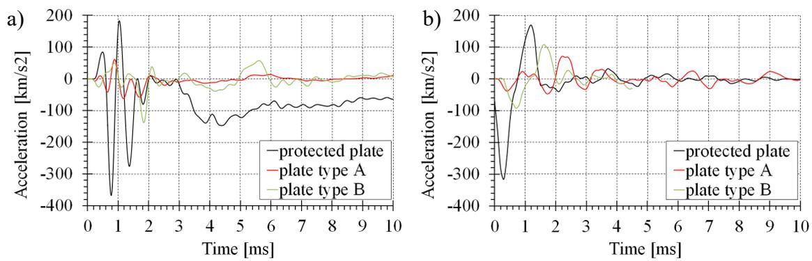
Fig. 8. Acceleration of the centre of the protected plate: a) experimental studies; b) numerical analysis
