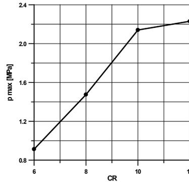
Fig. 12. Influence of compression ratio (CR) on the cycle maximum
