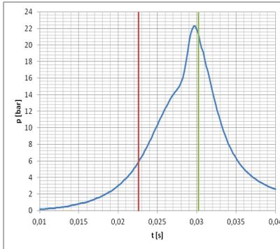
Fig. 11. High-speed waveforms of pressure in combustion chamber as a function of burning time: CR=12:1; IT= $50^{\circ}$  CABTDC
