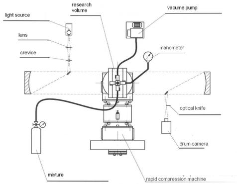
Fig. 3. Schematic of the optical system
