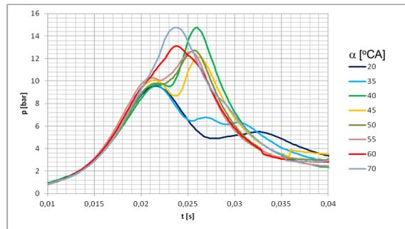
Fig. 8. High-speed waveforms of pressure in combustion chamber as a function of burning time: CR= 8:1;  $IT= 20^\circ$  to  $70^\circ$  BTDC
