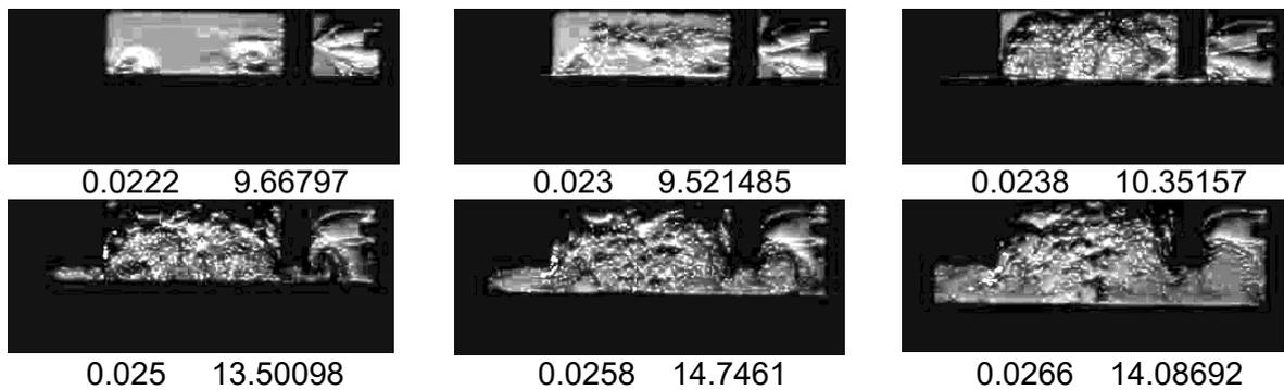
Fig. 7. Combustion process development in combustion chamber model:  $V_p=28\%$ , CR= 8:1;  $IT=40^\circ$  CABTDC
