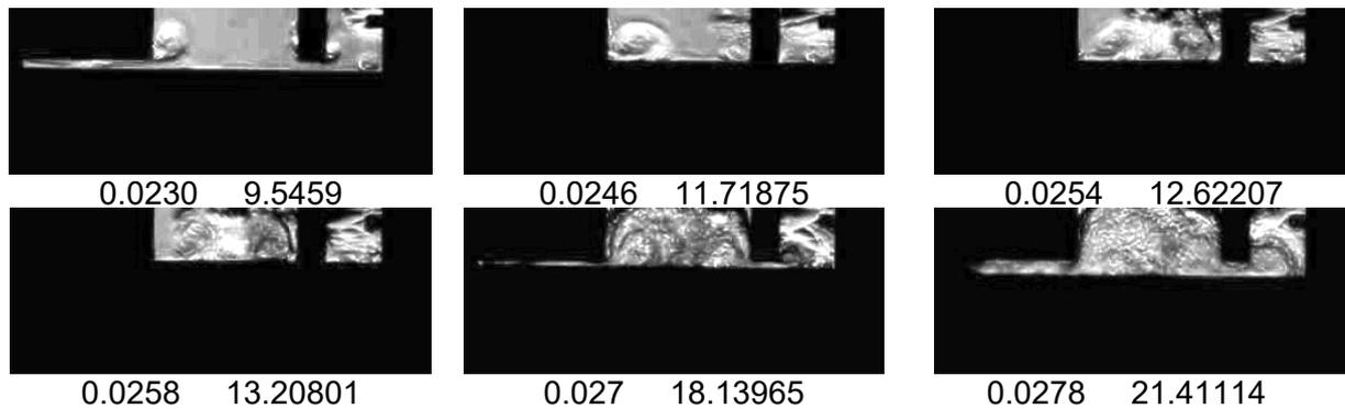
*Fig. 9. Combustion process development in combustion chamber model:  $V_p=28\%$ ,  $CR=10:1$ ;  $IT=40^0$  CABTDC*
