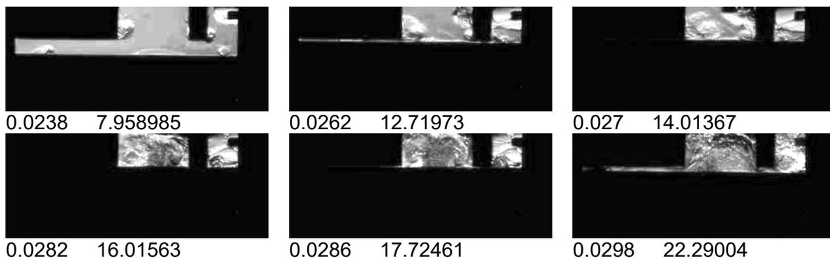
*Fig. 10. Combustion process development in combustion chamber model:  $V_p=28\%$ ,  $CR=12:1$ ;  $IT=50^0$  CABTDC*
