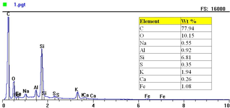
Fig. 3. Characteristic X-ray spectrum and chemical composition obtained for the surface layer of carbon nanotubes covering the bearing surface of the piston
