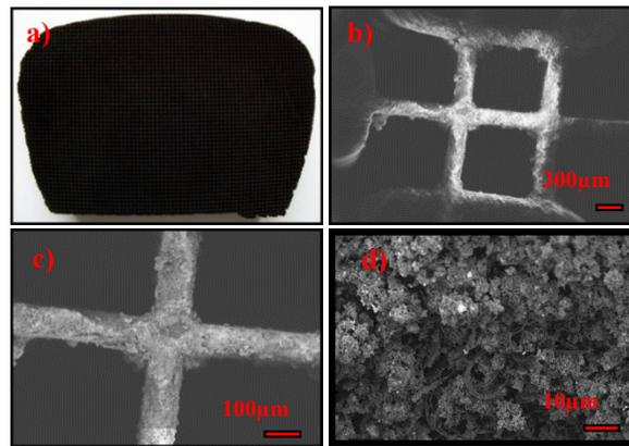
Fig. 5. Experimental catalytic reactor carrier ready to be fitted in the engine exhaust; a) the macroscopic image, b, c, d) Images recorded using a transmission electron microscope LEO 922A [21]
