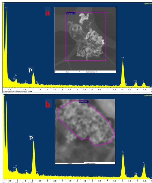
Fig. 7. The surface composition study – X-ray spectrum of areas presented in the pictures (EDX); a) sample with a side length of about 3 microns, b) irregular surface area selected from photo (a) [21]
