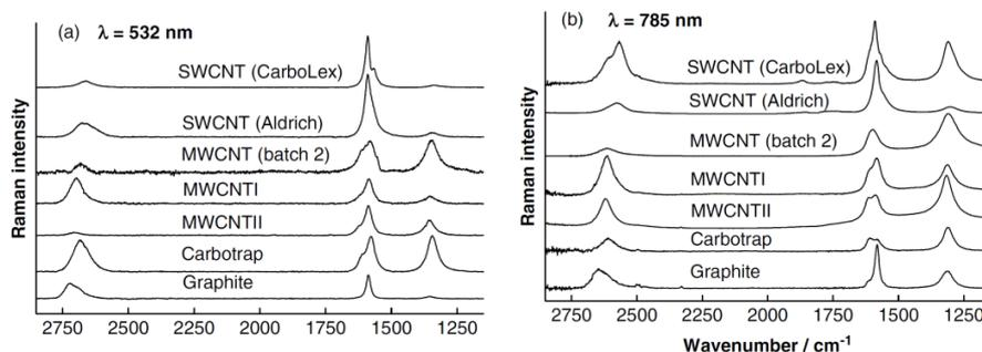
Fig. 4. Raman spectra obtained for the various allotropic forms of carbon for different excitation wavelengths (a: 532 nm; B: 785 nm) [13]
