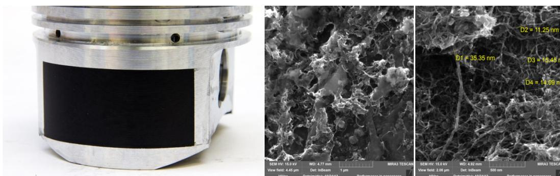
Fig. 2. The piston-bearing surface coated with carbon nanotubes layer; the pictures in macro scale and from scanning microscope obtained for sample from piston, which was dismantled from the engine after the researches at the test stand, were finished [15]
