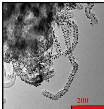
Fig. 6. The images obtained by HRTEM, showing single nanotubes on the surface of the reactor; on the surface of the nanotubes platinum nanoparticles are visible
