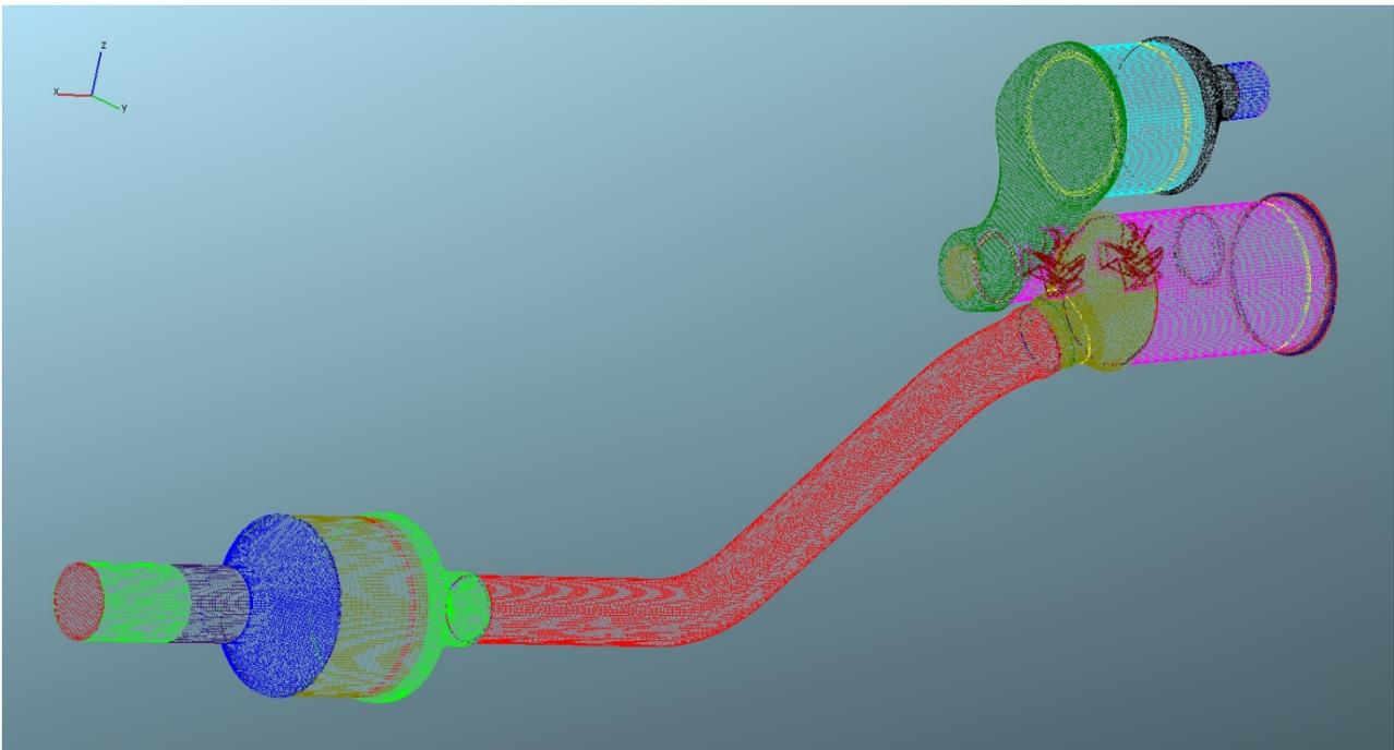
Fig. 4. Compact concept of SCR system in HD application
