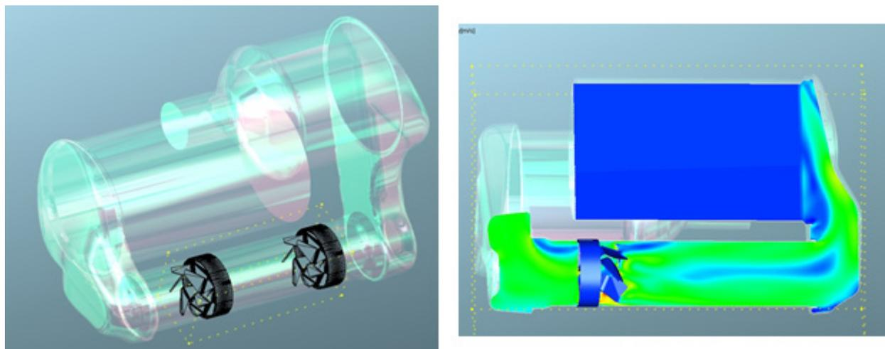
Fig. 5. Mixer models for CFD tests, on the left the two stage, on the right one stage mixer concept
