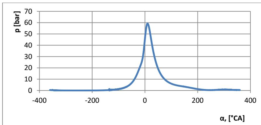
Fig. 10. Average pressure displacement chart (30 cycles of engine work), ignition timing:  $20^\circ$  before TDC
