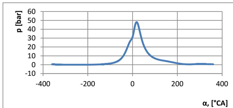
Fig. 7. Average pressure displacement chart (30 cycles of engine work), ignition timing: 110 before TDC
