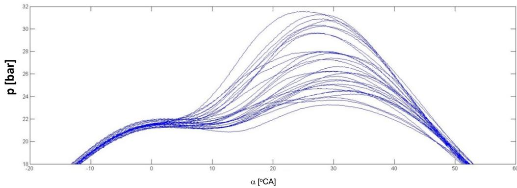
Fig. 5. Pressure displacement chart for 30 cycles (mixture no. 21)
