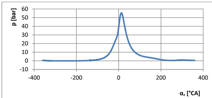
Fig. 9. Average pressure displacement chart (30 cycles of engine work), ignition timing:  $17.5^\circ$  before TDC
