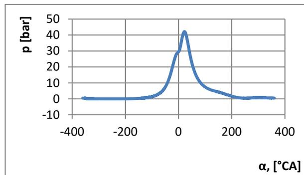
Fig. 6. Average pressure displacement chart (30 cycles of engine work), ignition timing: 8.5° before TDC
