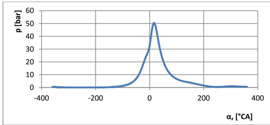
Fig. 8. Average pressure displacement chart (30 cycles of engine work), ignition timing:  $14.5^\circ$  before TDC
