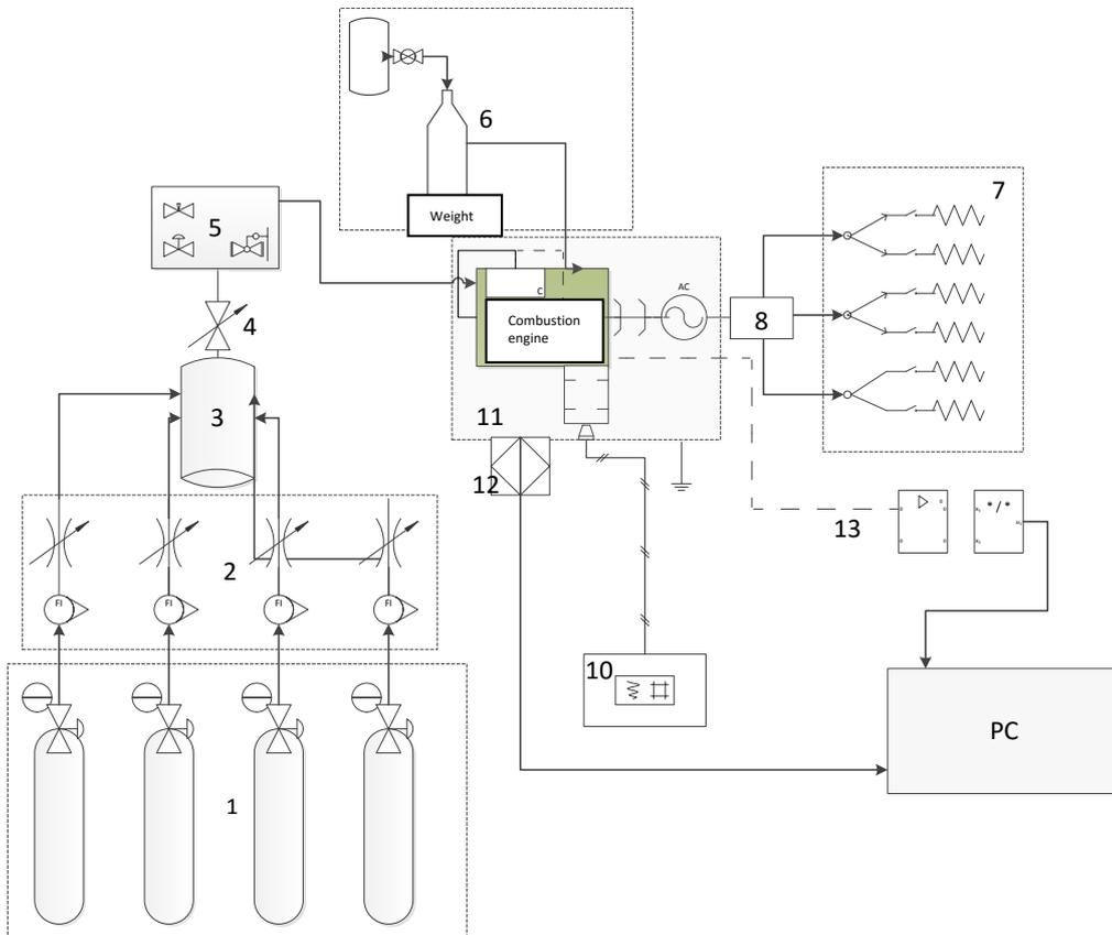
Fig. 2. Scheme of engine test stand
