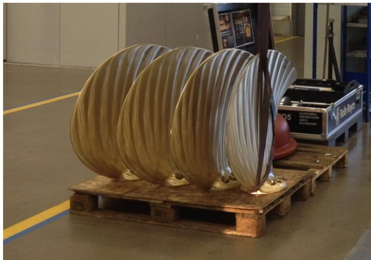
Fig. 7. Wing thruster after finishing abrasive treatment
