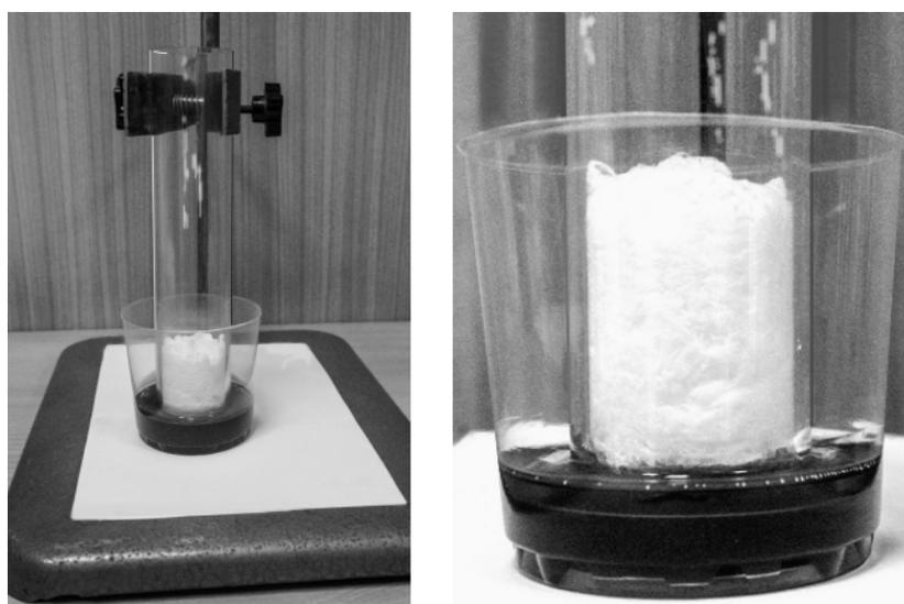
Fig. 2. The way of contacting of sorbent with oil
