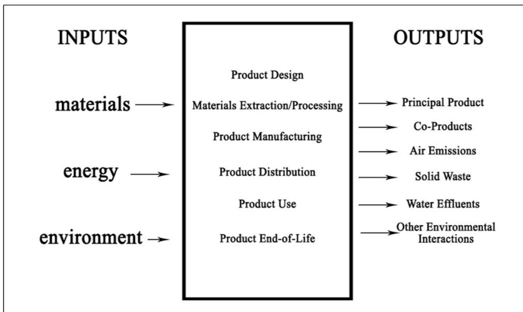
Fig. 2. Schematic structure of the LCA
