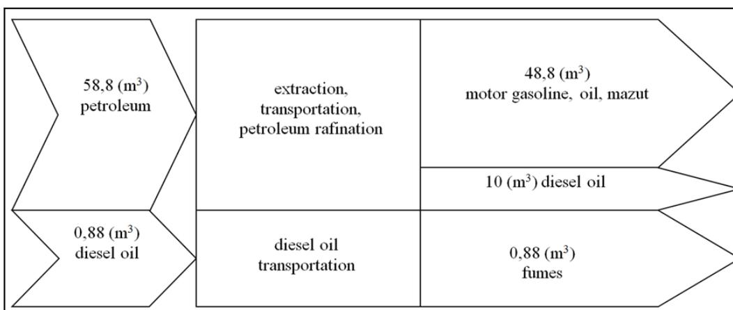
Fig. 5. The balance of raw material sourcing 10,000 litres of diesel oil
