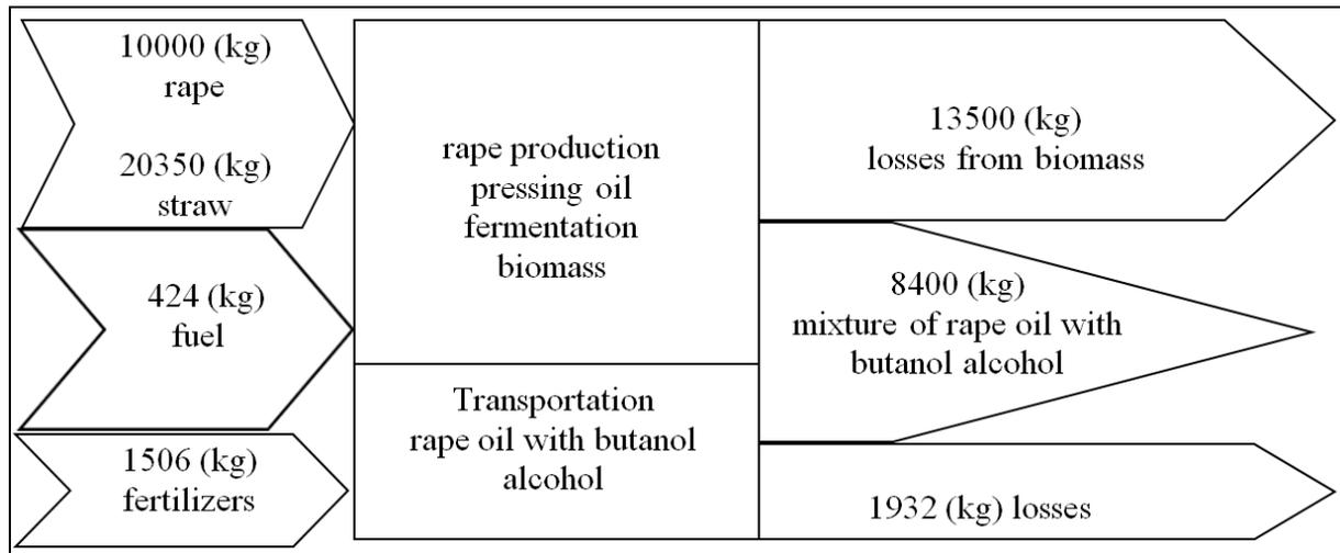
Fig. 6. The balance of the materials necessary to production 10000 litres of a mixture of rape oil and butanol alcohol (2:3 ratio)
