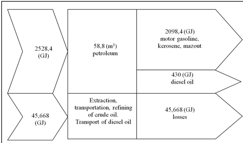
Fig. 3. The energy balance of the life cycle of diesel oil
