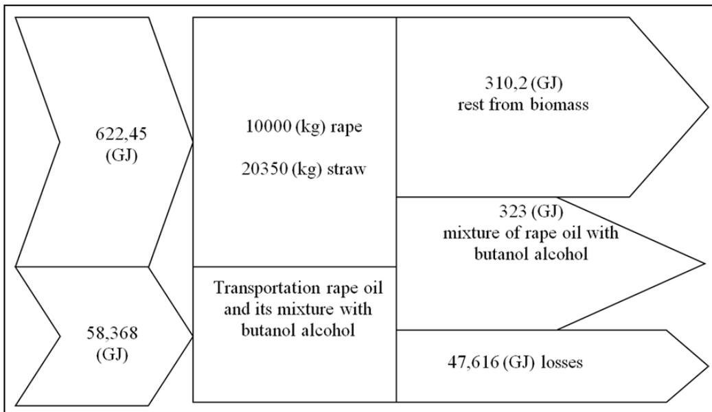
Fig. 4. The energy balance of the life cycle of rape oil mixed with butyl alcohol (ratio 2:3)
