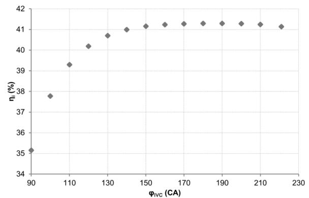
Fig. 10.  $\eta_i$  vs. IVC
