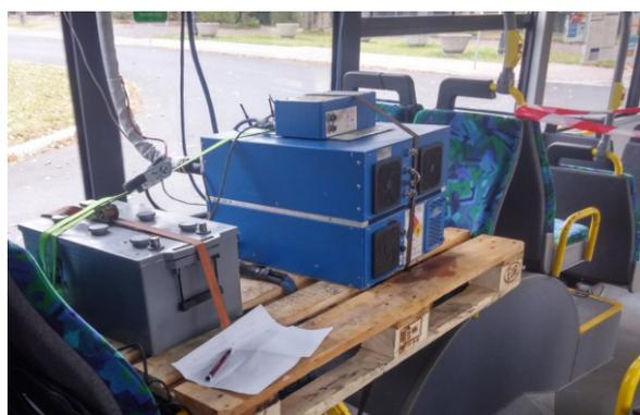
Fig. 9. Mobile device Semtech DS to measurement of exhaust emission pollutants under real conditions
