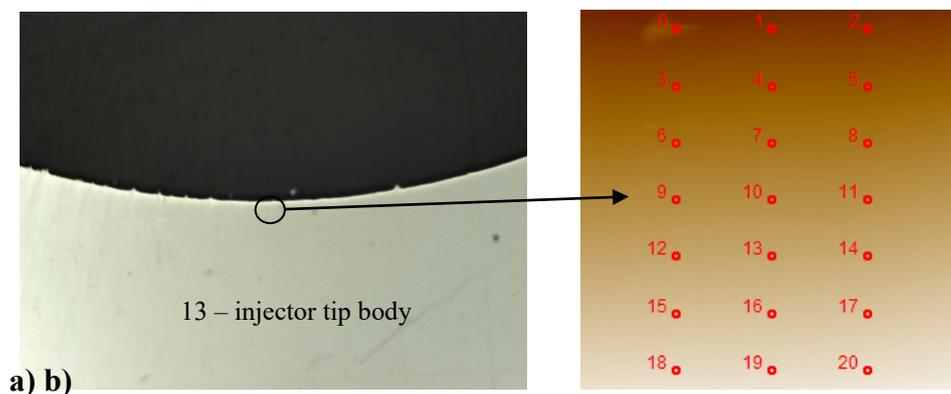
Fig. 2. The view of the investigated sample: a) an enlarged view – injector tip body (used), b) distribution of the measuring points
