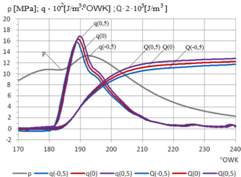
Fig. 6. Effect of TDC position errors on waveforms heat release characteristics  $q$  i  $Q$  low-speed marine diesel engine RTA76. The error value TDC (GMP in degrees rotation of the crankshaft) given in brackets
