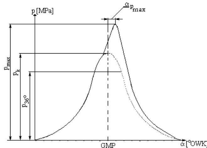
Fig. 2. Indicator diagram obtained from the electronic indicator and its characteristic values:  $p_{max}$  – the maximum combustion pressure,  $p_k$  – compression pressure,  $p_{36^\circ}$  (or  $p_{exp}$ ) – expansion pressure read 36 degrees of crankshaft rotation after TDC,  $\alpha_{p_{max}}$  – angle after TDC obtain maximum pressure in the cylinder
