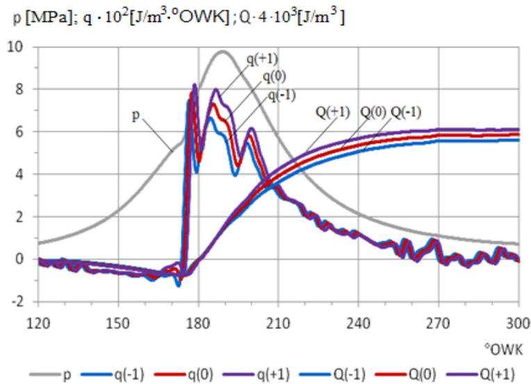
Fig. 5. Effect of TDC position errors on waveforms heat release characteristics  $q$  i  $Q$  medium-speed marine diesel engine A25/30. The error value TDC (GMP in degrees rotation of the crankshaft) given in brackets
