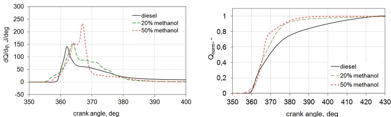
Fig. 3. Heat release rate ( $dQ/d\phi$ ) and accumulative heat release ( $Q$ ), (injection timing: 8.5 deg before TDC)
