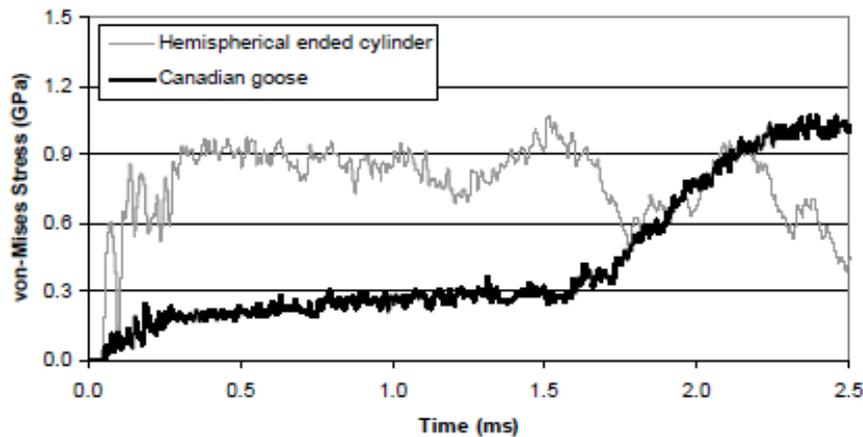
Fig. 4. Equivalent von-Mises stress (centre of panel target) predicted for the impact of a multi-material model, compared to the hemi-spherical ended cylinder [17]
