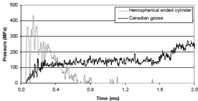
Fig. 3. Stagnation pressure (centre of panel target) predicted for the impact of a multi-material bird model, compared to a hemi-spherical ended cylinder [17]
