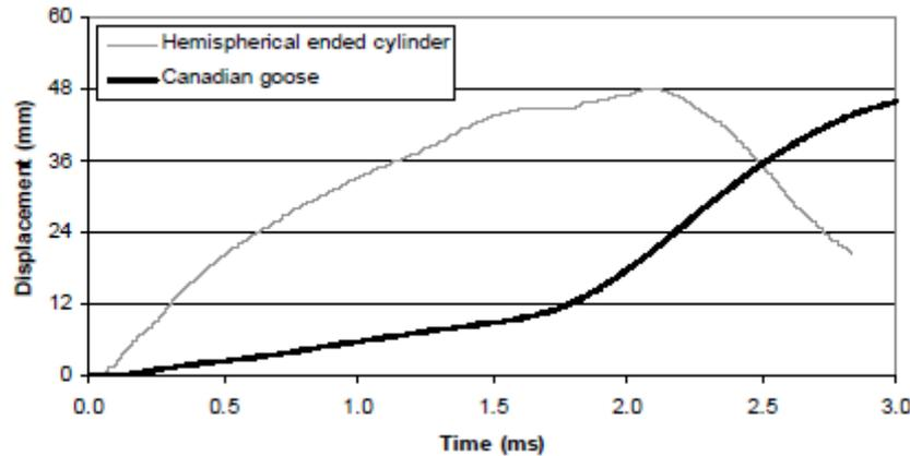
Fig. 5. Resultant displacement (centre of panel target) predicted for the impact of a multi-material model, compared to the hemi-spherical ended cylinder [17]
