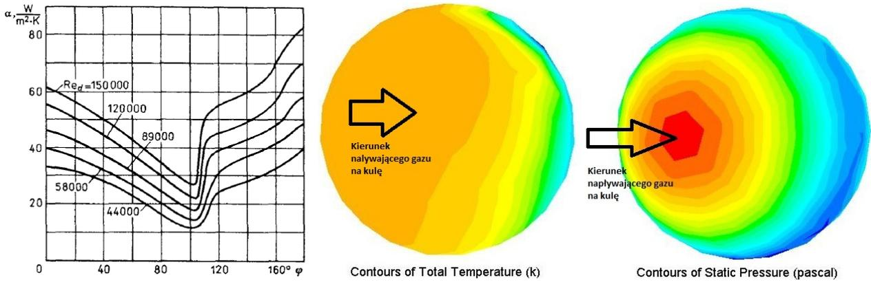
Fig. 2. The local distribution of heat transfer coefficients on the sphere [1] and exemplary distribution of temperature and pressure on the sphere during flow around
