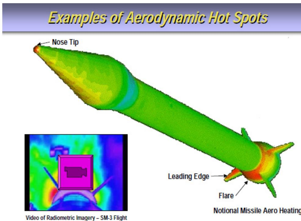
Fig. 6. Example of temperature distribution on rocket body [2]
