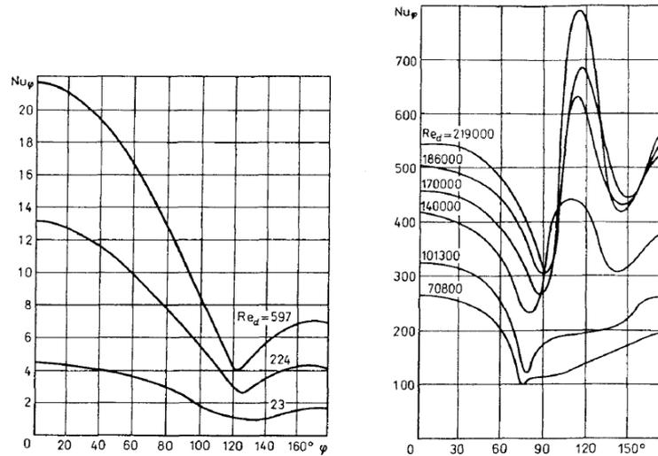
Fig. 3. Distribution of Nusselt numbers for different velocities of flow around roll [1]
