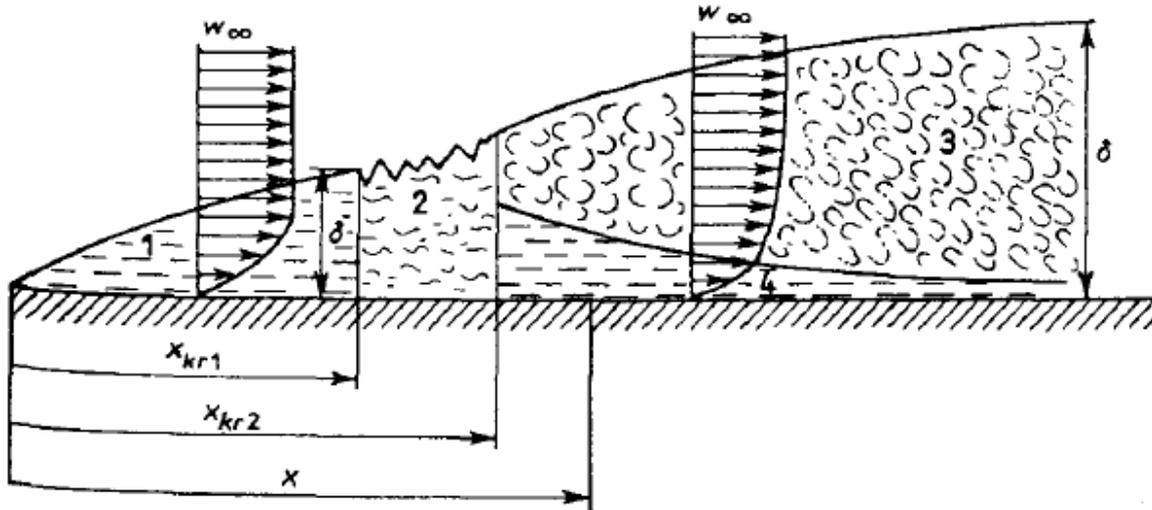
Fig. 1. Boundary layer at flow around the surface [1]
