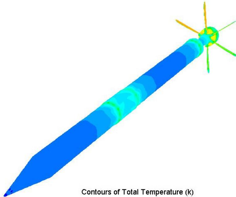
Fig. 9. Distribution of temperature field on body of rocket
