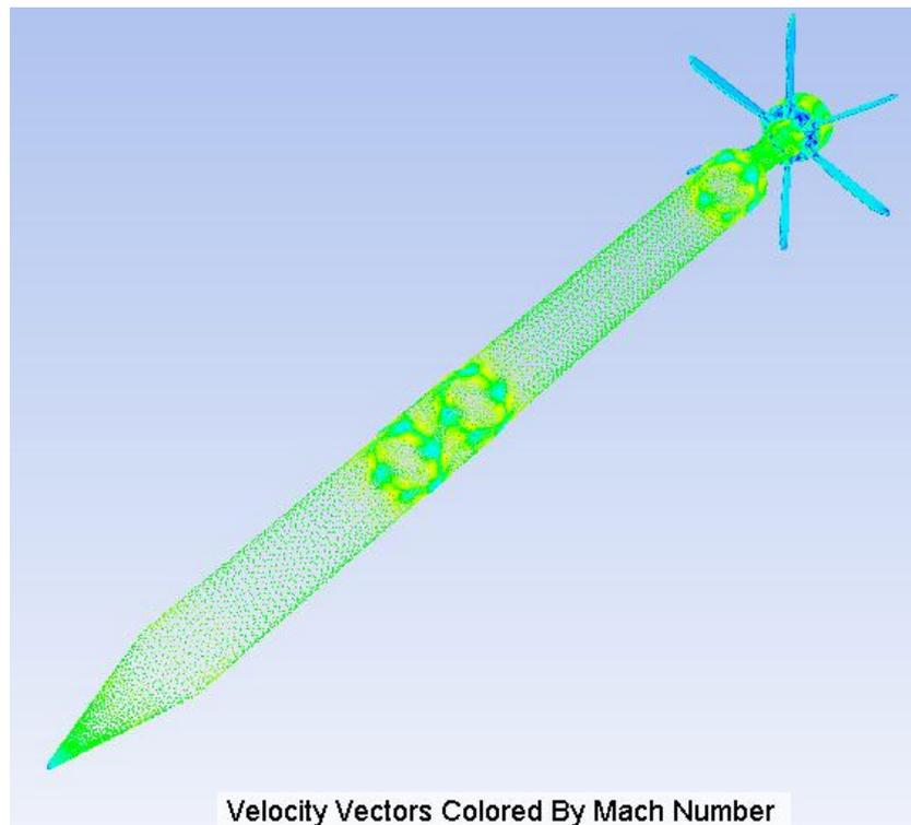
Fig. 8. Distribution of Mach number on body of rocket
