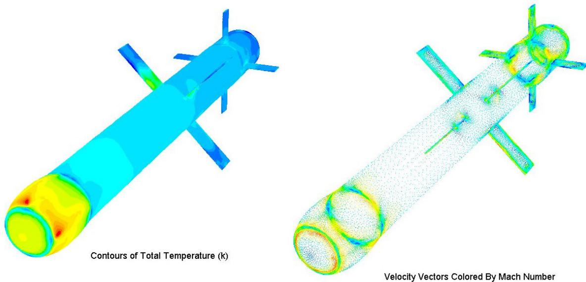
Fig. 10 Distribution of temperature field and velocity vectors on ground-ground rocket
