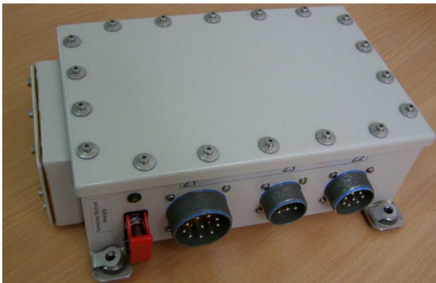
*Fig. 8. MUR-2 Microprocessor starting device*
