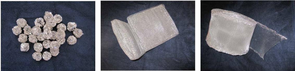
Fig. 13. Elements used to fill tanks to protect against explosion
