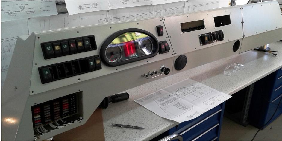
*Fig. 4. The ON-13 Driver's Dashboard*
