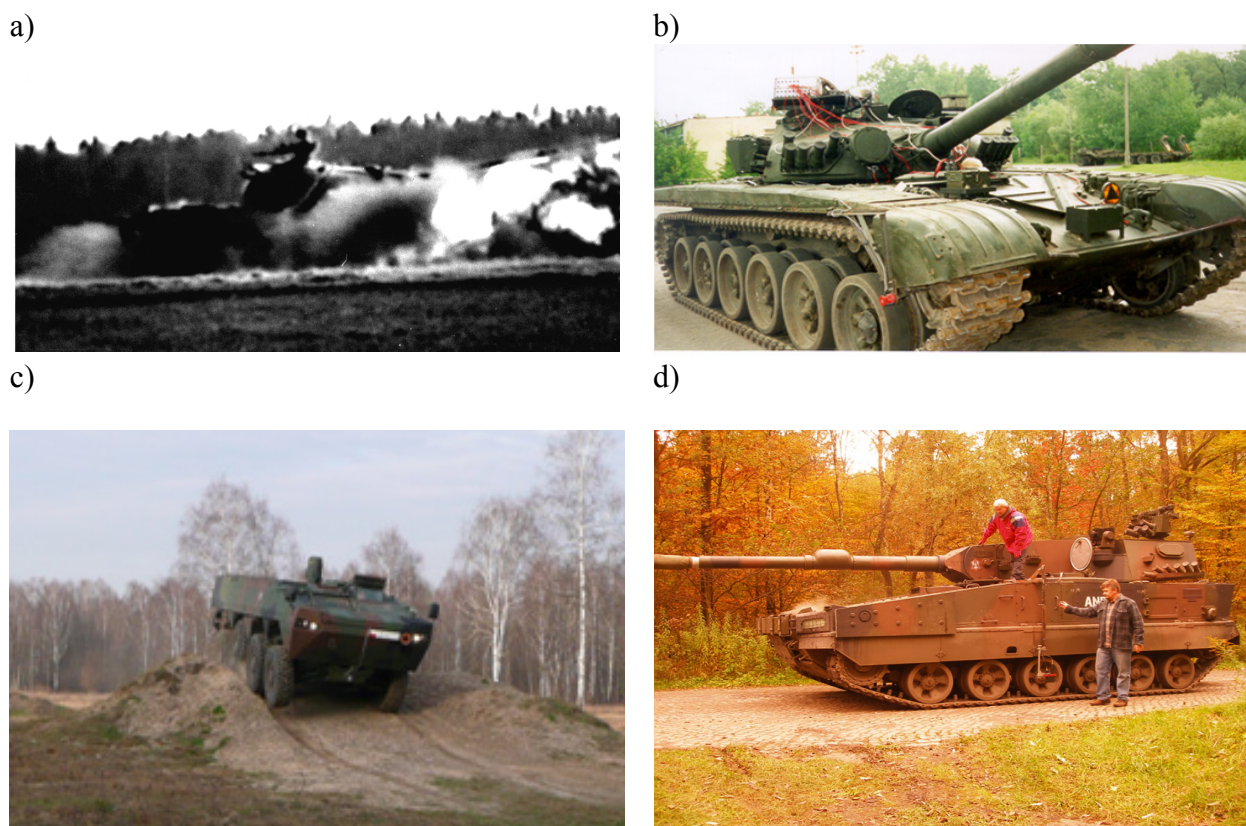
Fig. 1. Military vehicles taking part in the experimental tests: a) a tank during explosion of a model explosive under its bottom; b) a tank during the armament stabilization system tests on the military training area; c) wheeled armoured carrier during off-road driving; d) a prototype ANDERS tank during road tests
