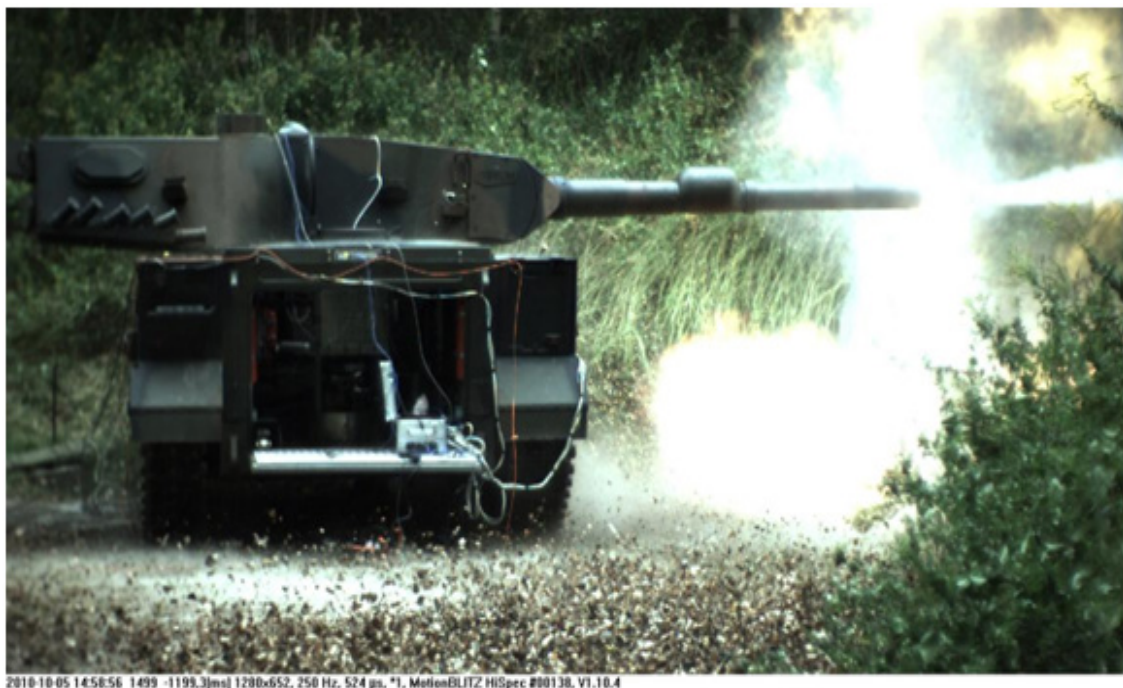
Fig. 3. Combat vehicle during firing from the main armament
