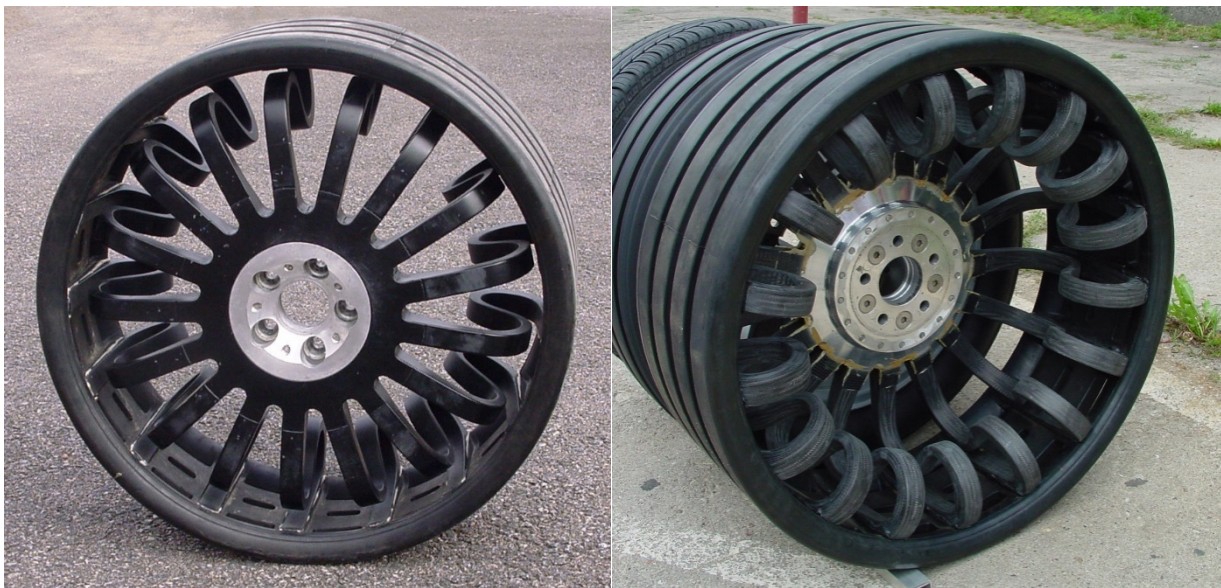
Fig. 6. View of a composite wheel developed in Sweden (Fig. from the archives of the Gdansk University of Technology)
