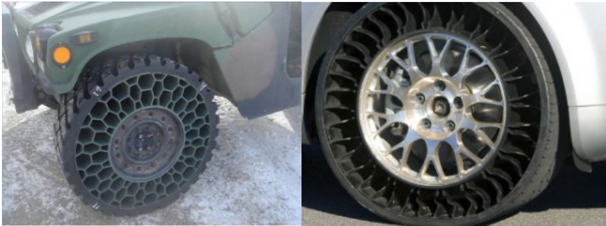
Fig. 5. View of vehicles with the Tweel system by Michelin (Fig. http://wkqsfm.com/featured/5932/michelin-tires-air-valve-stems )
