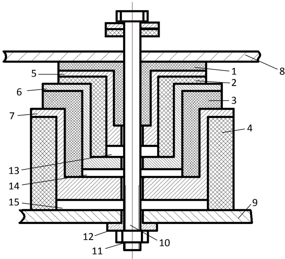
*Fig. 3. Scheme of proposed engineering solution of vibroisolator*
