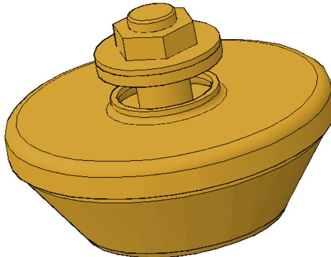
*Fig. 1. Cabin's vibroisolator of tractors DT and VT series*
