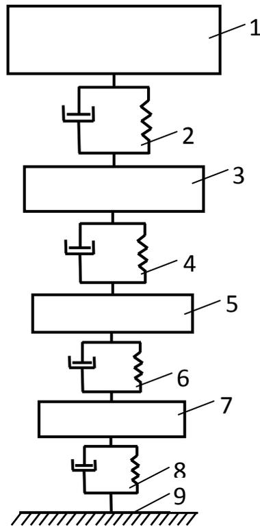
Fig. 4. Scheme of four-mass oscillating system
