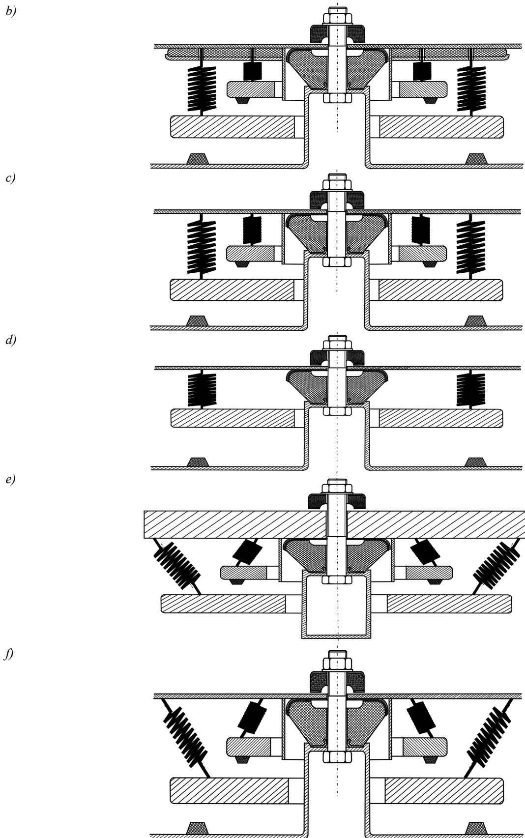
Fig. 2. Schemes of dynamic vibroisolators: a) – three masses in line and conic springs; b) – three parallel masses, elastomer and standard vibroisolator; c) – two parallel masses and standard vibroisolator; d) – one mass and standard vibroisolator; e) – two parallel masses, cabin's mass, standard vibroisolator and springs installed angularly; f) – two parallel masses, standard vibroisolator and spring installed angularly
