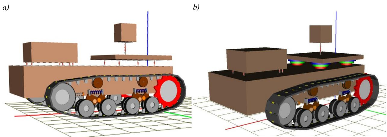
Fig. 5. Three-dimensional model: a) – with standard damper; b) – with dynamic dampers
