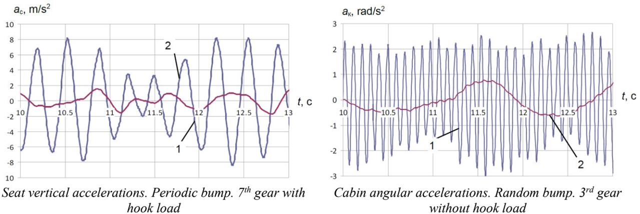
Fig. 6. Examples of comprising oscillograms
