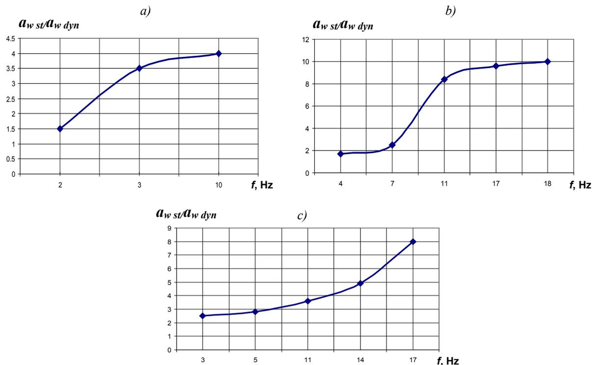
Fig. 7. Comparison of efficiency of cabin suspension with standard and dynamic vibroisolators: a – decreasing of seat vertical acceleration amplitudes; b – decreasing of cabin vertical acceleration amplitudes; c – decreasing of seat and cabin angular acceleration amplitudes
