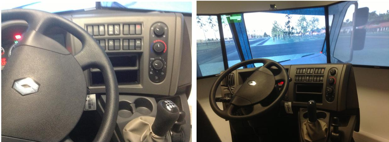
Fig. 3. Replicating the National Fire Service vehicle driver's station with the view generated by the virtual simulator [3]
