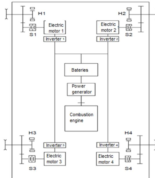
Fig. 4. Diagram of the hybrid drive concept
