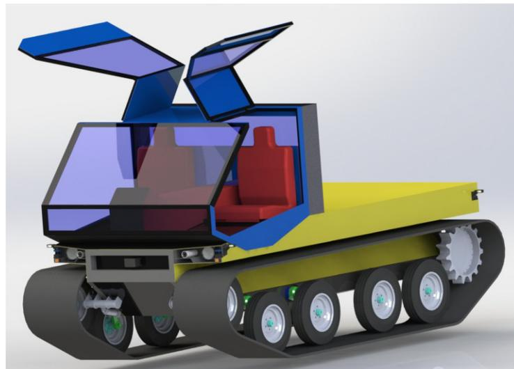
Fig. 8. The cab concept of the WIPH vehicle
