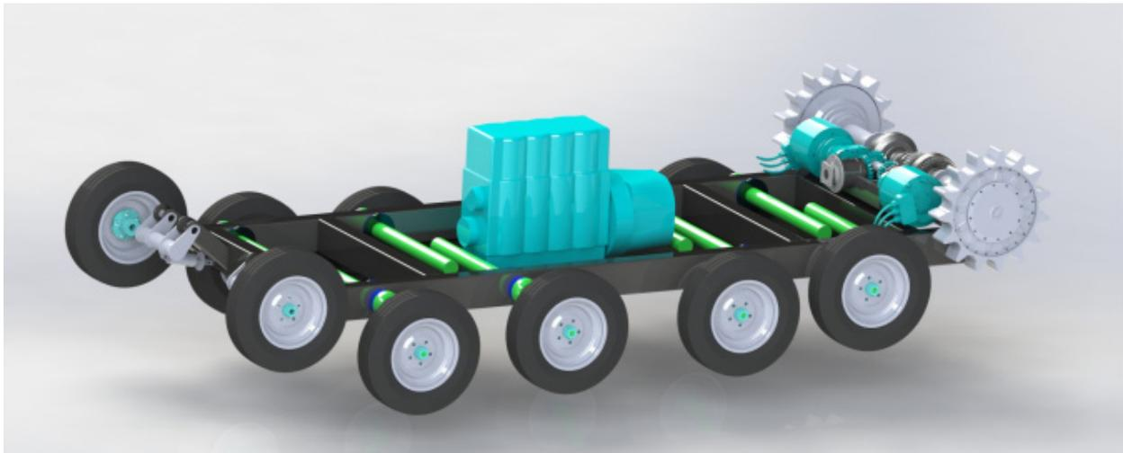
Fig. 5. The configuration of the WIPH vehicle wheels and steering system
