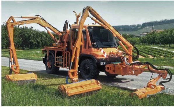
Fig.1. UNIMOG U500 Vehicle
