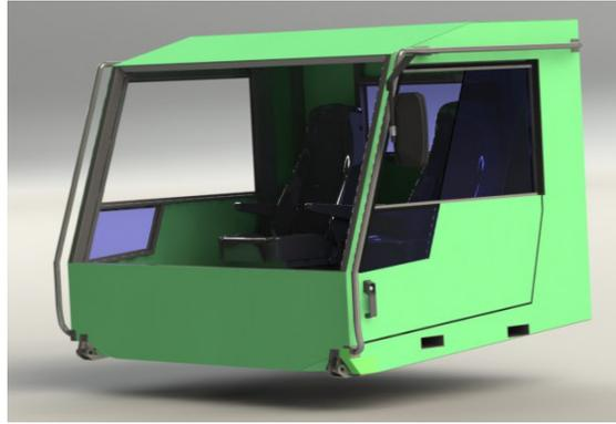
Fig. 9. Model of the WIPH vehicle cab
