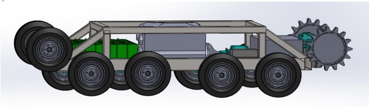
Fig. 6. Suspension configuration with a) lowered and b) raised first pair of road wheels
