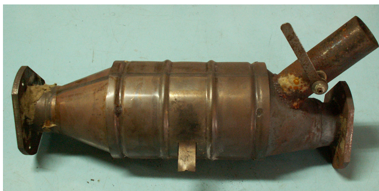
Fig. 1. Catalytic converter with an eccentric cone, with connecting flanges and nozzle to be mounted electric heater (platinum-palladium catalytic reactor Pt/Pd – number of ducts: 500 cpsi, load: 1g/dm 3 , ratio Pt:Pd/2:1)
