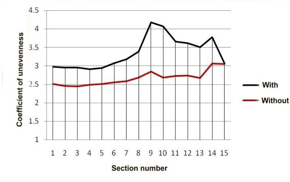
Fig. 5. Change of coefficient  $k_H$  on areas at longitudinal motion without hook load
