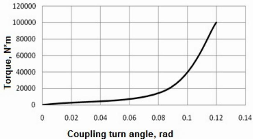
Fig. 2. Coupling elastic characteristic
