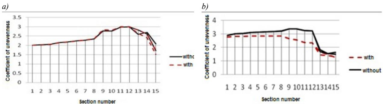
Fig. 6. Change of  $k_H$  on areas at steady turn: a-speed is 0.56 m/s, turn radii is 5 m; b – speed is 1.67 m/s, turn radii is 5 m
