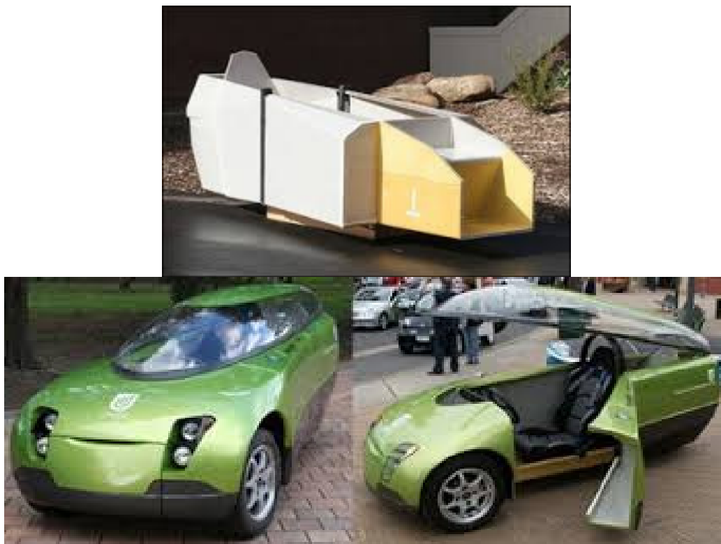
Fig. 6. Supporting structure and complete ultra-light vehicle (2)
