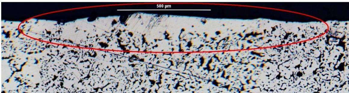
Fig. 4. Cross-section of the path made with  $CO_2$  laser
