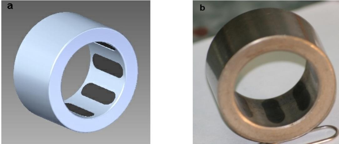
Fig. 3. Paths made with  $CO_2$  laser beam on the sliding surface of  $\varnothing 25/\varnothing 35 \times 20$  mm sleeve: numerical model, b) real sleeve
