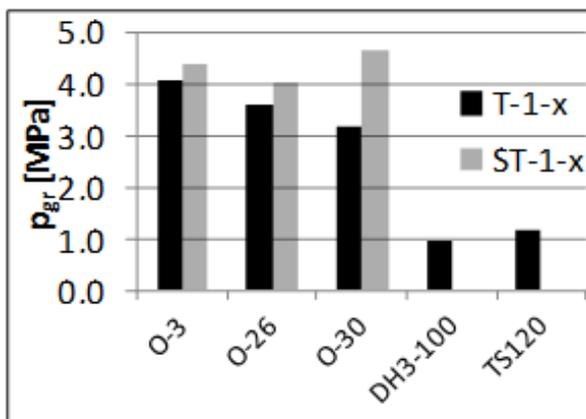
Fig. 7. Influence of the micro-segments of ST-1-x sleeves on  $p_{gr}$  increase at 1000 rpm
