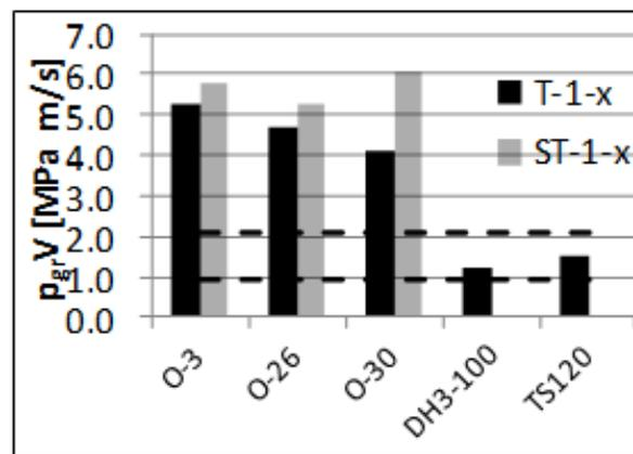
Fig. 8. Influence of the micro-segments of ST-1-x sleeve on increasing of  $p_{gr} \cdot v$  product at 1000 rpm
