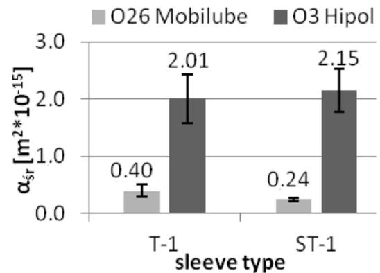
Fig. 14. The comparison of average oil permeability of the tested sleeves for 0-3 (Hipol) and 0-26 (Mobilube) oils
