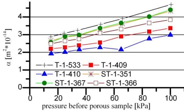
Fig. 11. Air permeability of standard (T-1-x) and new generation (ST-1-x) sleeves
