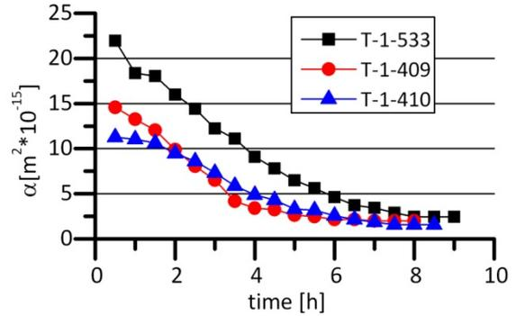
Fig. 12. Oil permeability of standard T-1-x sleeves (Hipol 15 F (O-3) oil)
