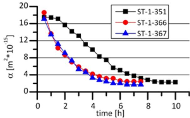
Fig. 13. Oil permeability of new generation ST-1-x sleeves (Hipol 15 F (O-3) oil)
