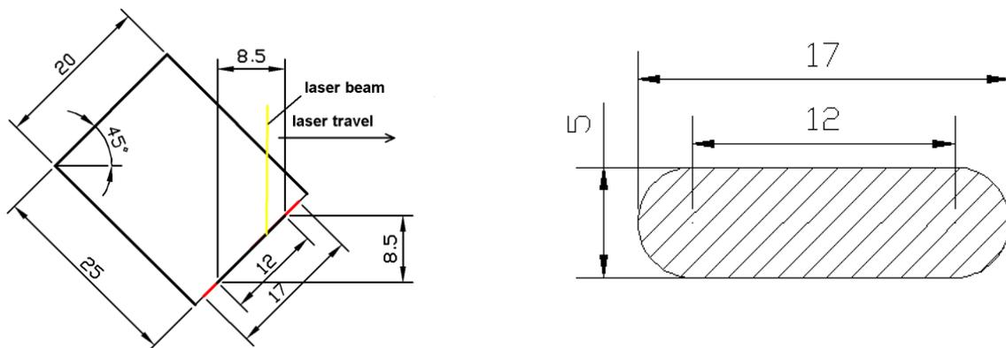
Fig. 1. Scheme of sleeve set-up in relation to the laser beam Fig. 2. Exemplary geometric dimensions of the path (micro-segment)
