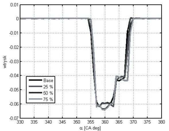
Fig. 9. Average injector coil current changes for  $N = 3000$  rpm,  $T = 1000$  Nm and different ester percentages in the used fuel
