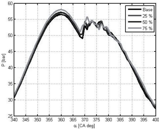
Fig. 6. Average cylinder pressure changes for  $N = 3000$  rpm,  $T = 100$  Nm and different ester percentages in the used fuel
