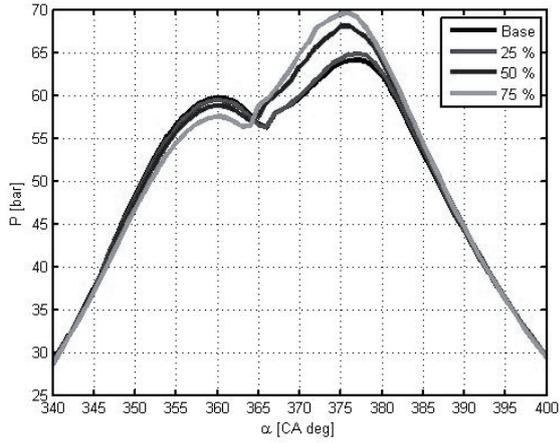
Fig. 4. Average cylinder pressure changes for  $N = 1500$  rpm,  $T = 150$  Nm and different ester percentages in the used fuel
