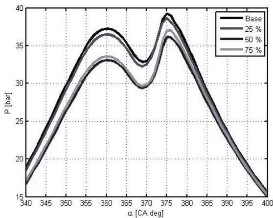
*Fig. 2. Average cylinder pressure changes for N = 1500 rpm, T = 50 Nm and different ester percentages in the used fuel*
