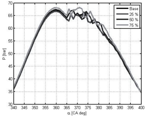
Fig. 7. Average cylinder pressure changes for  $N = 3000$  rpm,  $T = 150$  Nm and different ester percentages in the used fuel
