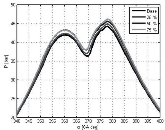
*Fig. 3. Average cylinder pressure changes for N = 1500 rpm, T = 100 Nm and different ester percentages in the used fuel*
