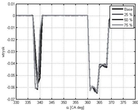
Fig. 8. Average injector coil current changes for  $N = 1500$  rpm,  $T = 100$  Nm and different ester percentages in the used fuel
