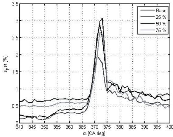
Fig. 10. Cylinder pressure signal standard deviation changes for  $N = 1500$  rpm,  $T = 50$  Nm and different ester percentages in the used fuel
