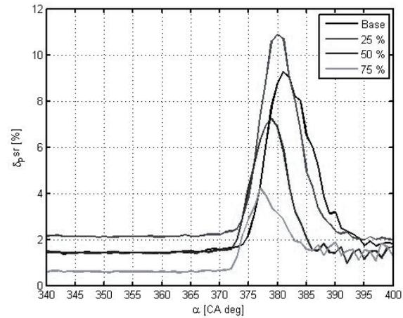
Fig. 11. Cylinder pressure signal standard deviation changes for  $N = 3000$  rpm,  $T = 50$  Nm and different ester percentages in the used fuel
