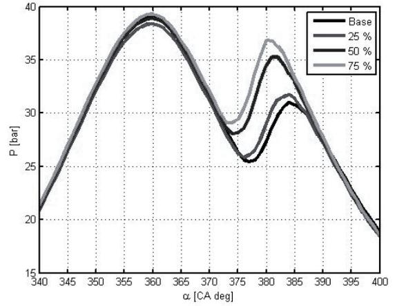
Fig. 5. Average cylinder pressure changes for  $N = 3000$  rpm,  $T = 50$  Nm and different ester percentages in the used fuel
