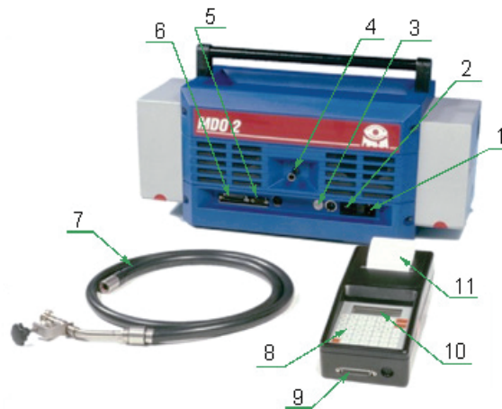
Fig. 3. Smokemeter MDO 2: 1 – power connection, 2 – main switch, 3 – lamp indicating that the device is ON/OFF, 4 – connection of the measuring probe, 5 – connection for data transfer, 6 – socket for the wire connecting the manual control panel with the central unit of MDO 2, 7 – wire connecting the probe with the central unit of MDO 2, 8 – alphanumeric keyboard of the manual control panel, 9 – connection of the wire connecting the control panel with the central unit, 10 – LCD display, 11 – paper
