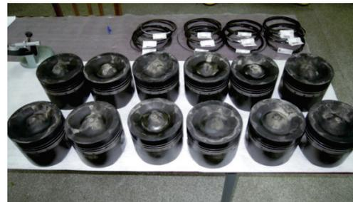
Fig. 4. Diesel engine pistons after the motor tests
