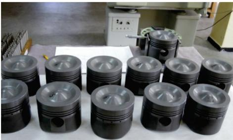
Fig. 3. Diesel engine pistons prior to motor tests
