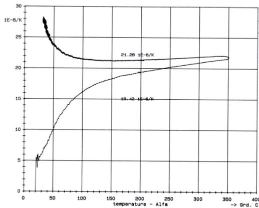
Fig.1.Changes of thermal expansion coefficient of raw state silumin alloy  $AlSi12Ni4Cu4Mg0.5CrMoWV$  during heating and cooling
