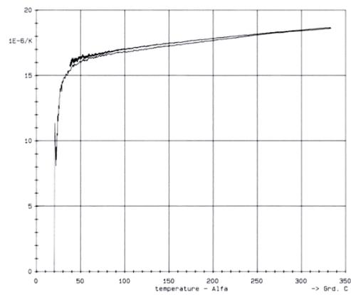
Fig. 2. Changes of thermal expansion coefficient of silumin alloy  $AlSi12Ni4Cu4Mg0.5CrMoWV$  after the heat treatment
