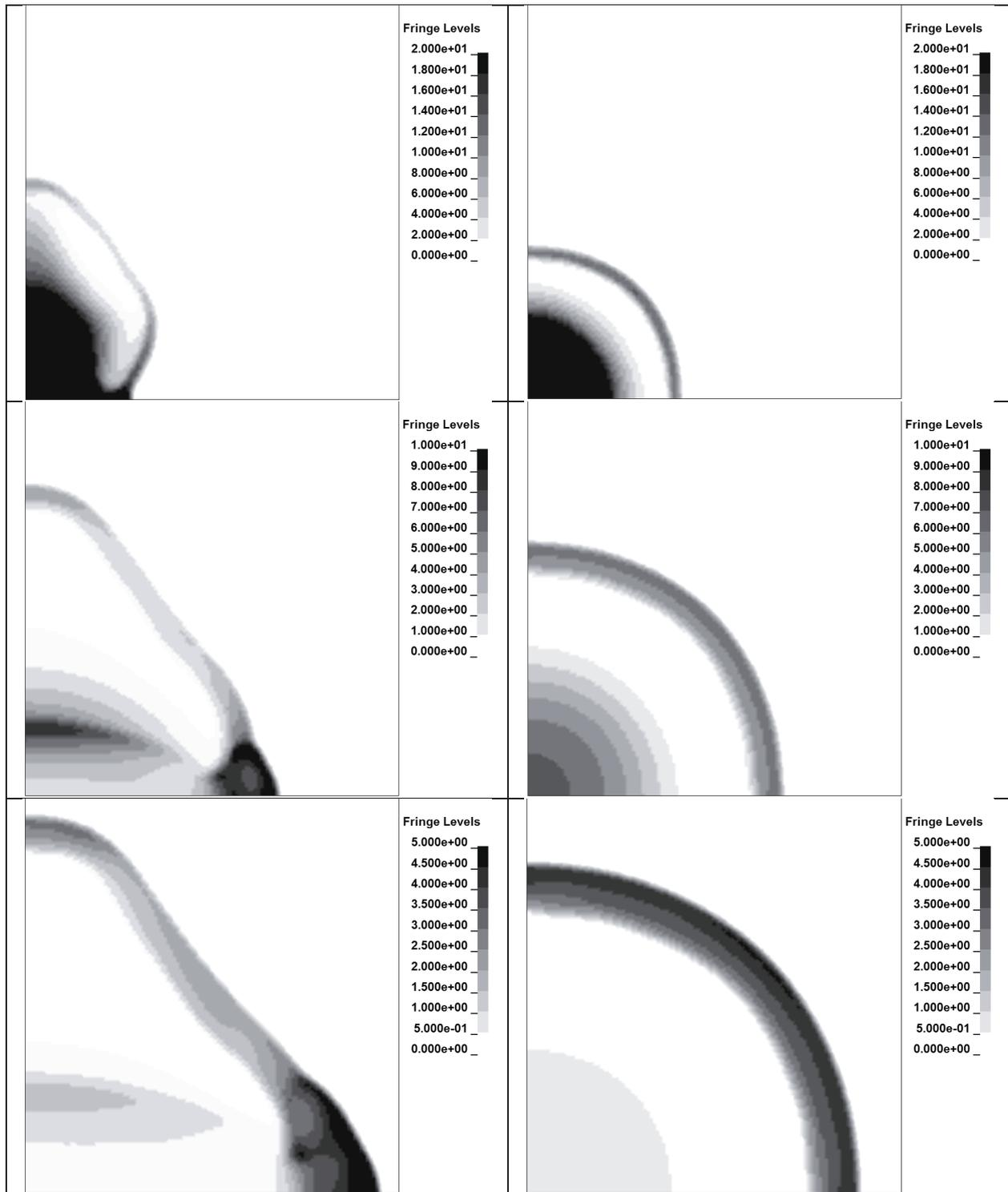
Fig. 3. Pressure wave propagation - cylindrical (left) and hemispherical shape (right) [MPa],  $t = 0.1; 0.2; 0.3$  ms
