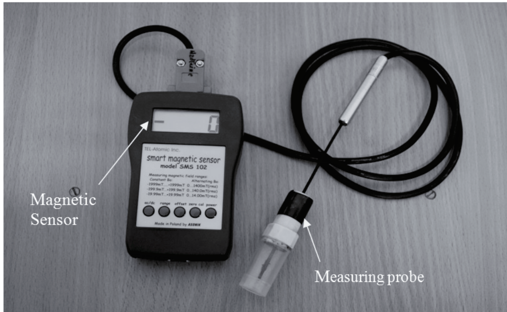
Fig. 3. Hall Effect Meter SMS102, together with the measuring probe
