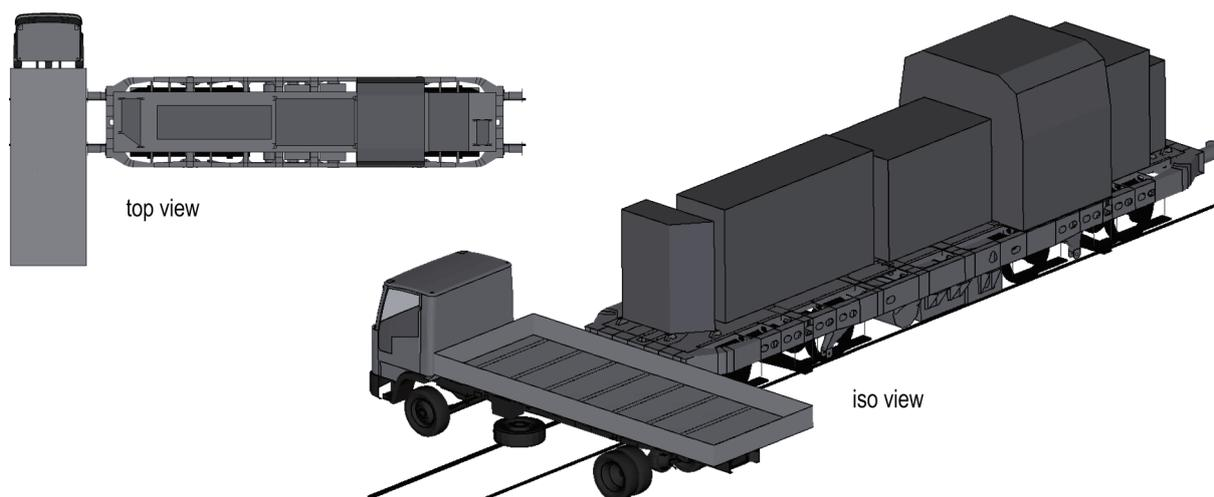
Fig. 1. FE model of the locomotive and the truck located on a level crossing – FE mesh not shown
