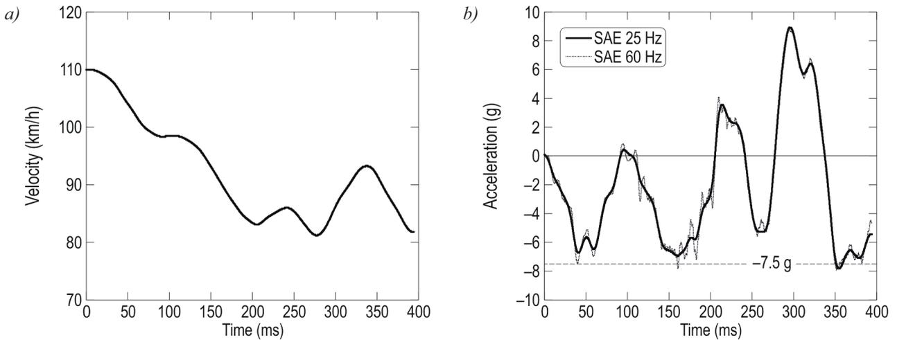
Fig. 3. Velocity (a) and acceleration (b) of the locomotive cab obtained from the FE analysis
