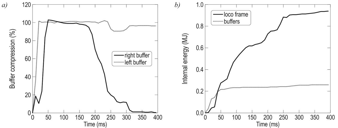
Fig. 7. Time history of buffers' compression (a) and internal energy of buffers and the locomotive frame (b) obtained from the FE analysis
