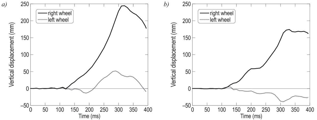
Fig. 6. Time history of vertical displacement of the axleboxes for the first (a) and the second (b) wheelset of the front bogie confirming a serious risk of the locomotive derailment
