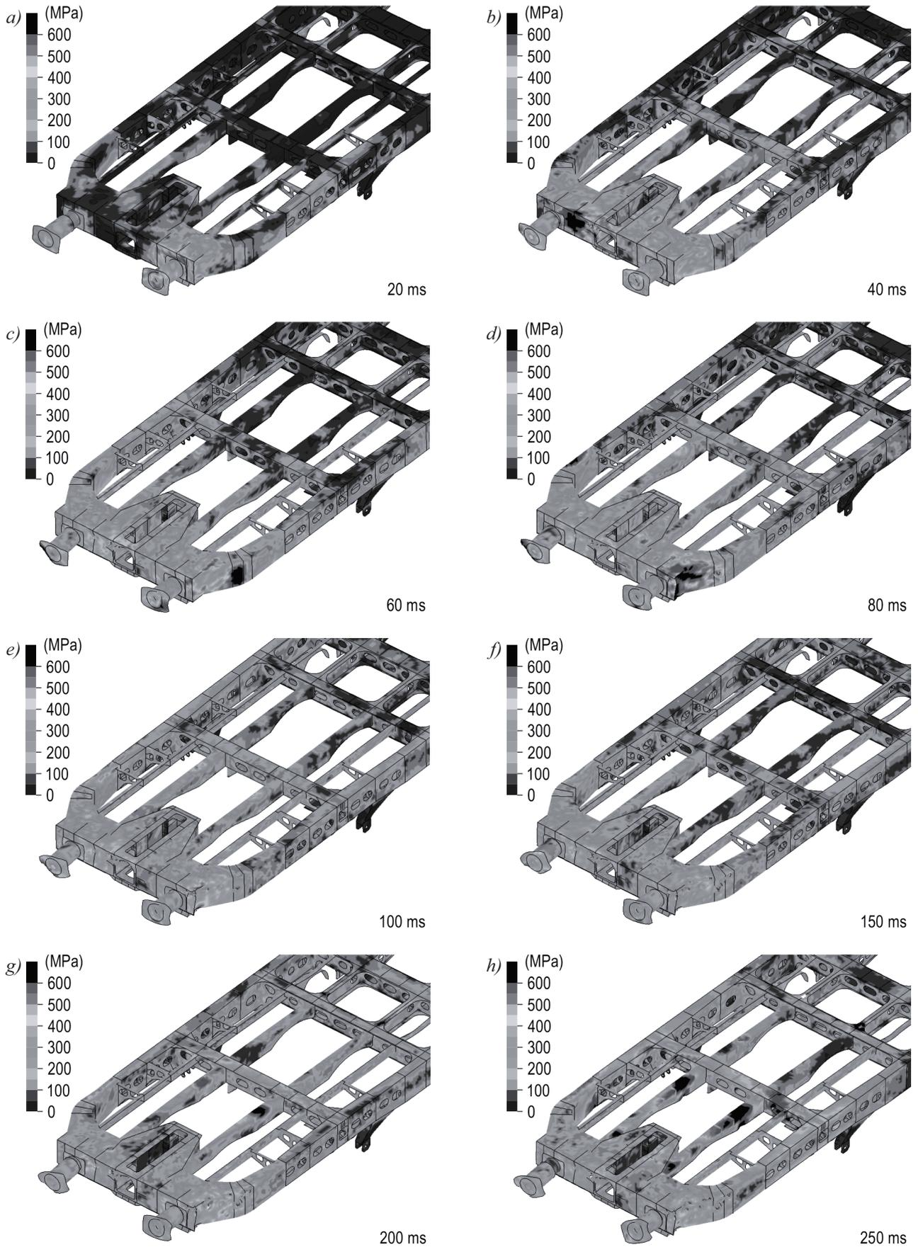
Fig. 8. Contours of the effective von Mises stress for the locomotive frame in selected moments of time: 20 ms (a), 40 ms (b), 60 ms (c), 80 ms (d), 100 ms (e), 150 ms (f), 200 ms (g), 250 ms (h)
