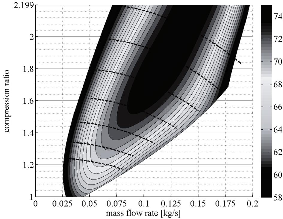
Fig. 3. KKK2464 compressor characteristics converted to the digital form (graph drawn for full range values of the contours)
