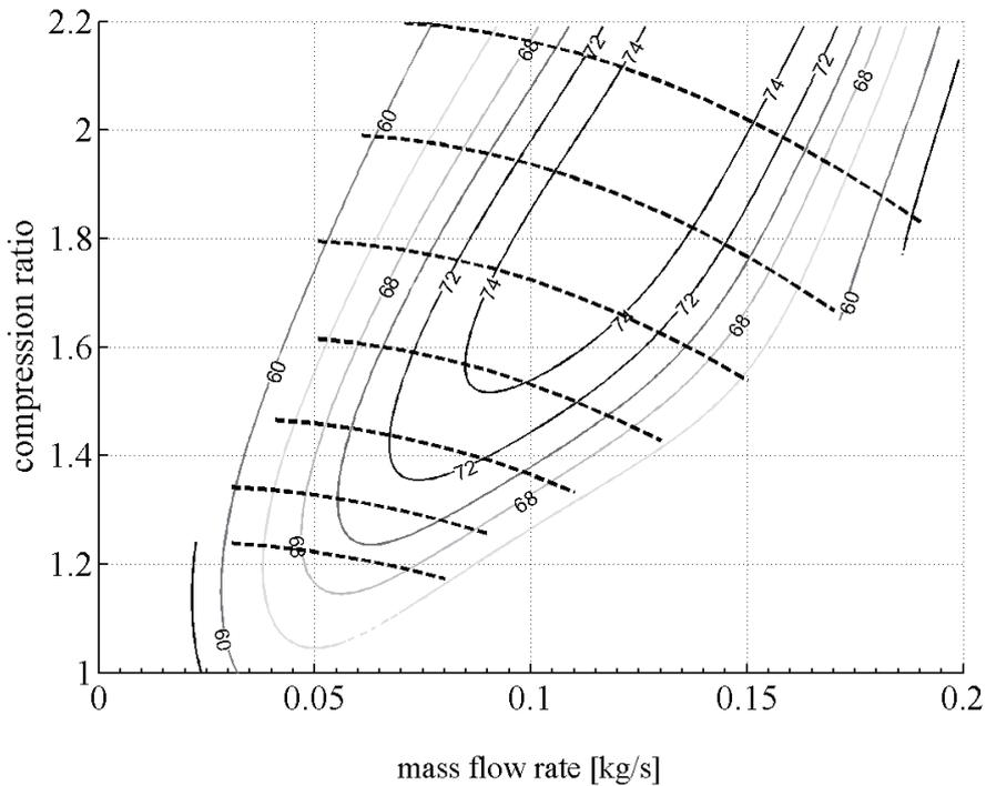
Fig. 2. Centrifugal compressor performance map [2]
