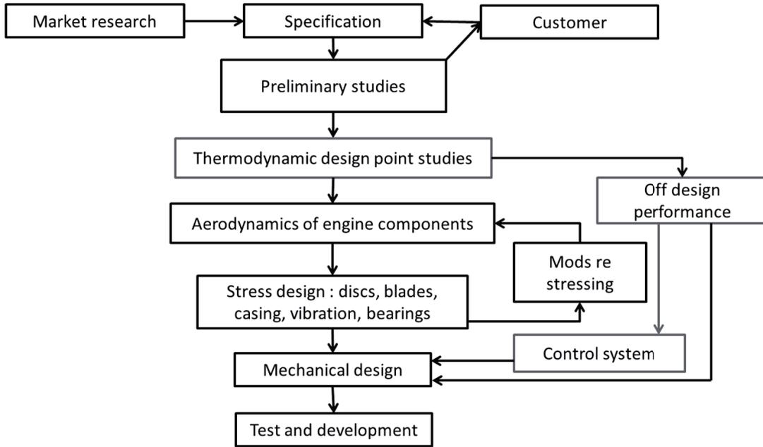
Fig. 1. PMDO gas turbine design steps [10]
