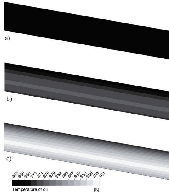
Fig. 11. Temperature distribution in slide conical bearing gap with relative eccentricity  $\lambda = 0.6$ , for  $L = 25$  mm and the lowest value of gap height: a)  $n_r = 500$  rpm, b)  $n_r = 3200$  rpm, c)  $n_r = 7200$  rpm
