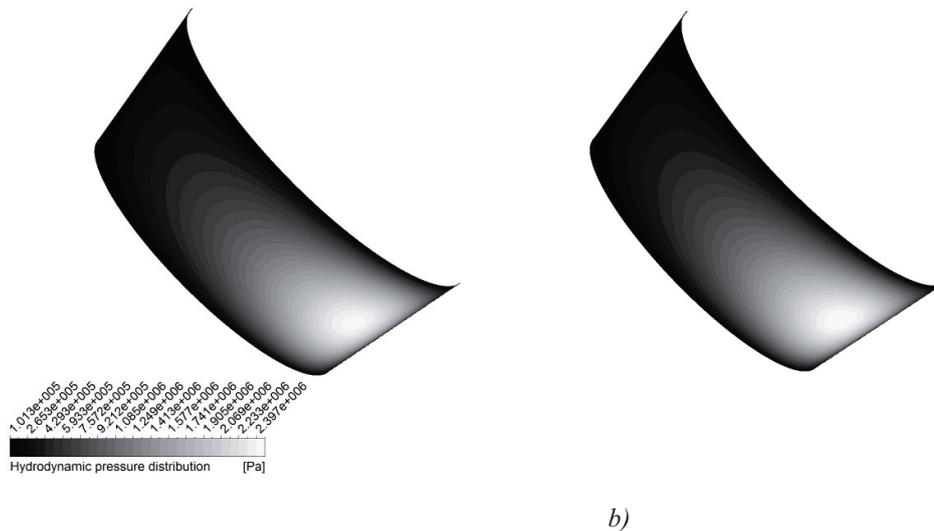
Fig. 8. Hydrodynamic pressure distribution in slide conical bearing;  $\lambda = 0.6$ ,  $n_r = 500$  rpm a) lubricated with non-Newtonian oil and including viscous heating, b) non-Newtonian isothermal lubrication
