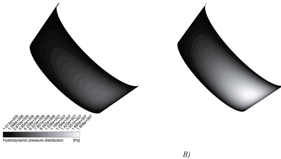
Fig. 7. Hydrodynamic pressure distribution in slide conical bearing;  $\lambda = 0.5$ ,  $n_r = 7200$  rpm a) lubricated with non-Newtonian oil and including viscous heating, b) non-Newtonian isothermal lubrication
