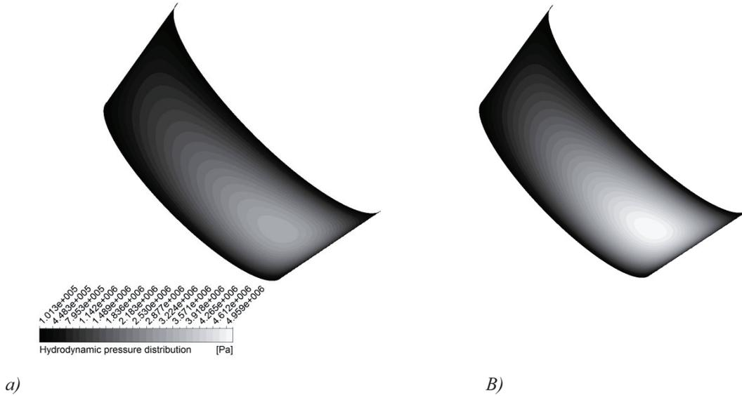
Fig. 3. Hydrodynamic pressure distribution in slide conical bearing;  $\lambda = 0.4$ ,  $n_r = 3200$  rpm a) lubricated with non-Newtonian oil and including viscous heating, b) non-Newtonian isothermal lubrication
