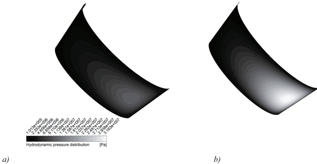
Fig. 10. Hydrodynamic pressure distribution in slide conical bearing;  $\lambda = 0.6$ ,  $n_r = 7200$  rpm a) lubricated with non-Newtonian oil and including viscous heating, b) non-Newtonian isothermal lubrication
