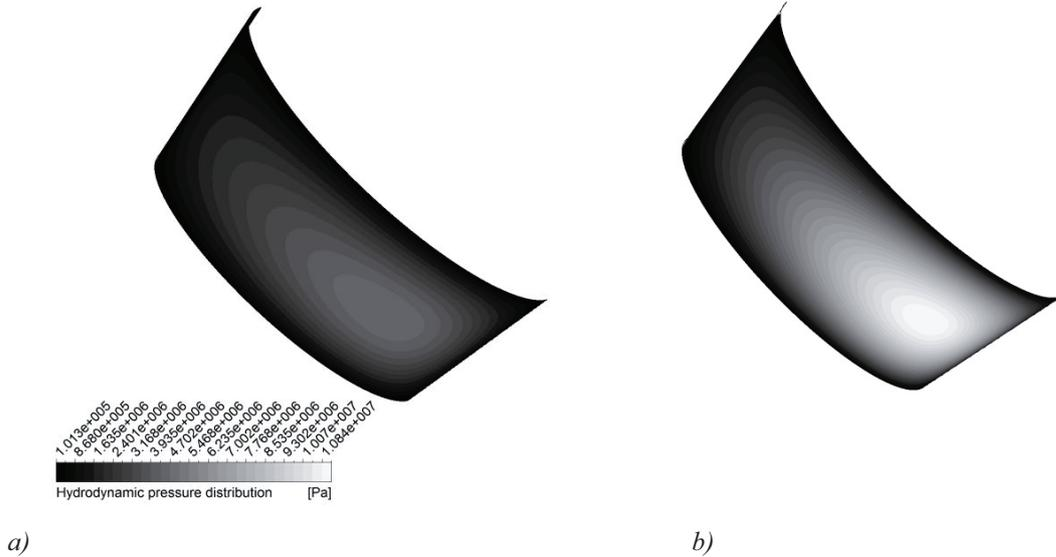
Fig. 4. Hydrodynamic pressure distribution in slide conical bearing;  $\lambda = 0.4$ ,  $n_r = 7200$  rpm a) lubricated with non-Newtonian oil and including viscous heating, b) non-Newtonian isothermal lubrication
