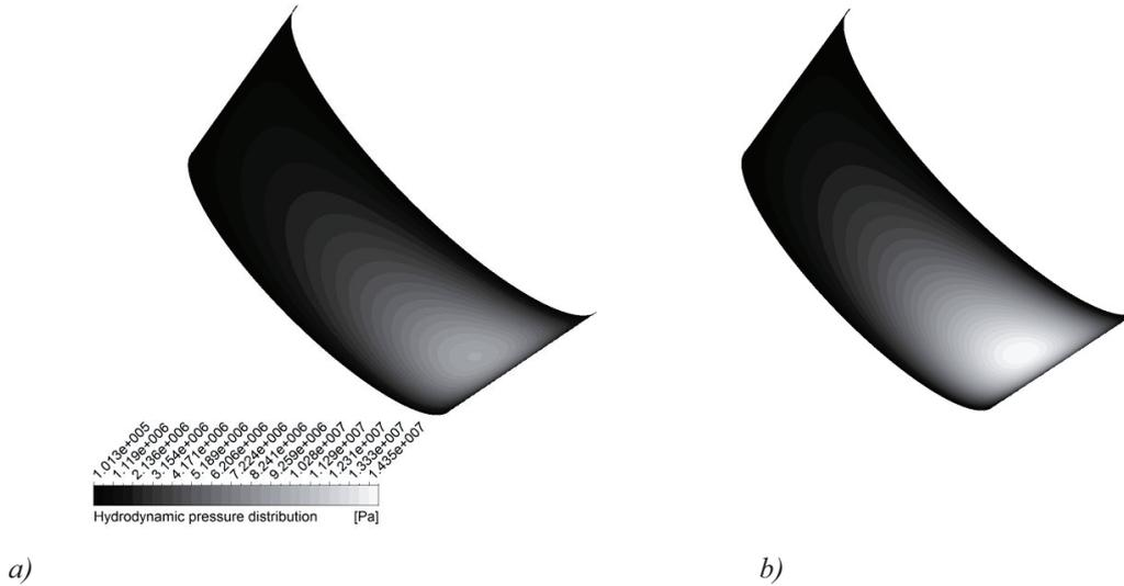
Fig. 9. Hydrodynamic pressure distribution in slide conical bearing;  $\lambda = 0.6$ ,  $n_r = 3200$  rpm a) lubricated with non-Newtonian oil and including viscous heating, b) non-Newtonian isothermal lubrication
