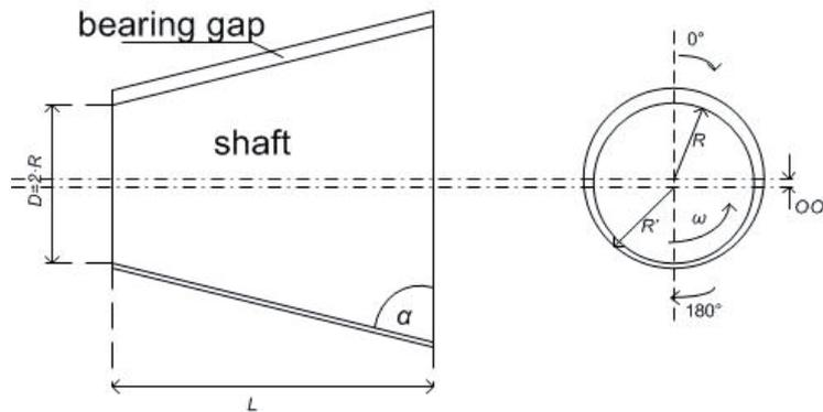
Fig. 1. The investigated bearing geometry
