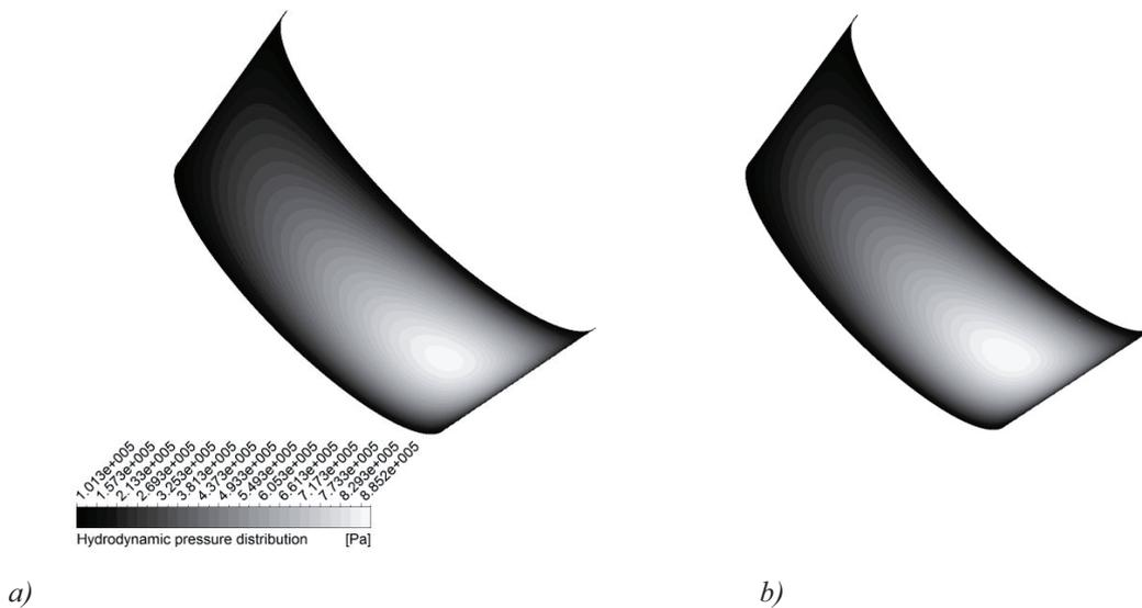
Fig. 2. Hydrodynamic pressure distribution in conical slide bearing;  $\lambda = 0.4$ ,  $n_r = 500$  rpm a) lubricated with non-Newtonian oil and including viscous heating, b) non-Newtonian isothermal lubrication
