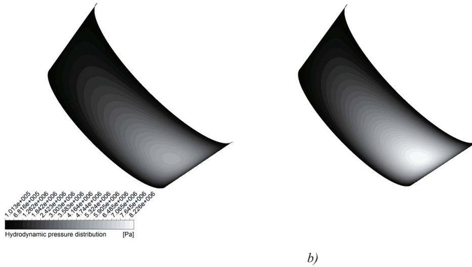
Fig. 6. Hydrodynamic pressure distribution in slide conical bearing;  $\lambda = 0.5$ ,  $n_r = 3200$  rpm a) lubricated with non-Newtonian oil and including viscous heating, b) non-Newtonian isothermal lubrication
