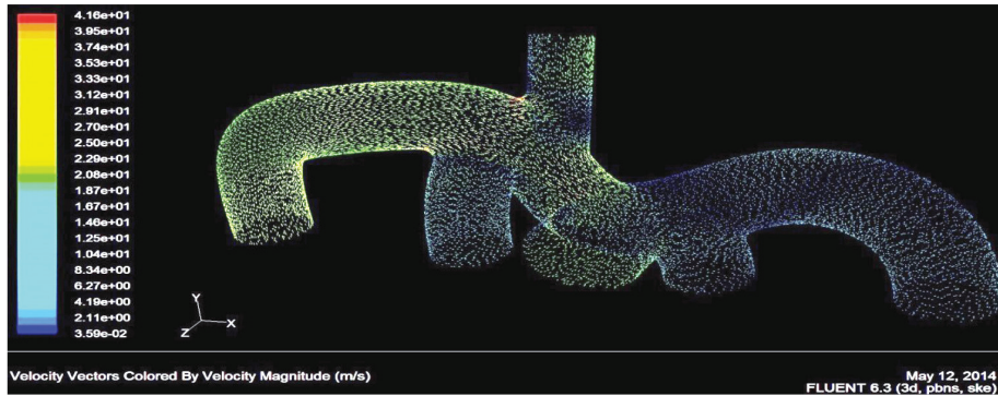
Fig. 9. Distribution of fluid velocity on the walls
