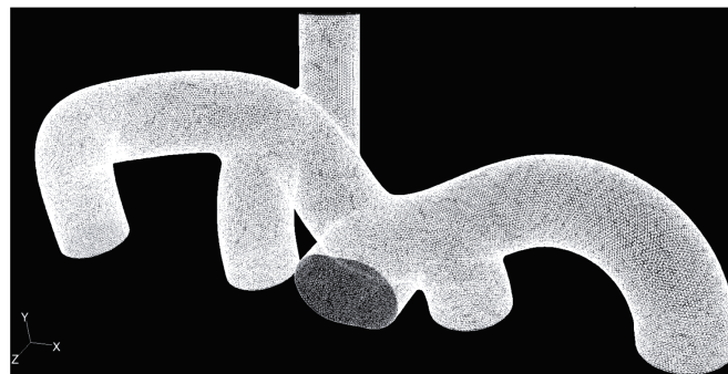
Fig. 3. Grid visualization of space limiting fluid volume in ANSYS FLUENT
