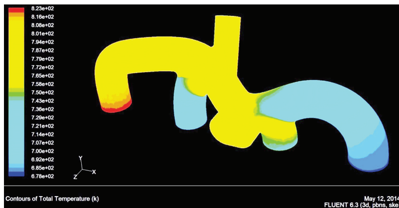
Fig. 8. The distribution of total temperature on the walls of exhaust manifold
