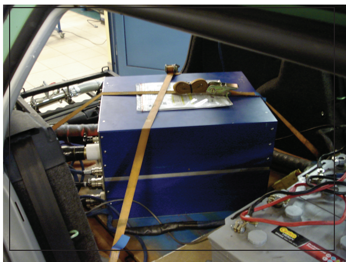
Fig. 3. Measuring equipment (PEMS type) mounted on the vehicle
