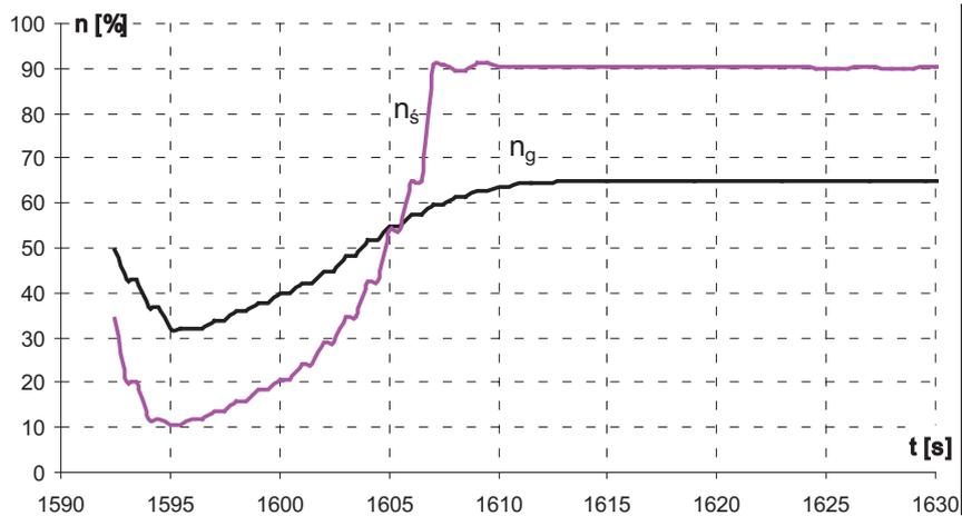
Fig. 17. Variations of the engine and airscrew rpm during the second restart
