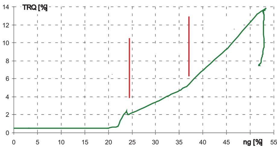
Fig. 5. Variations of the engine torque as a function of the turbine generator rpm during the engine start-up
