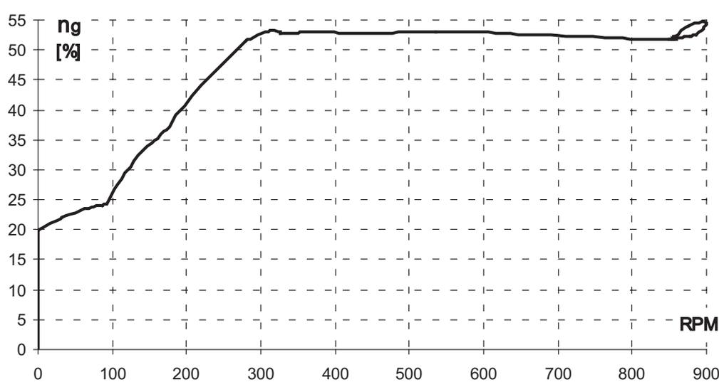
Fig. 4. Characteristic curves for variation of the turbine generator rpm as a function of the airscrew rpm
