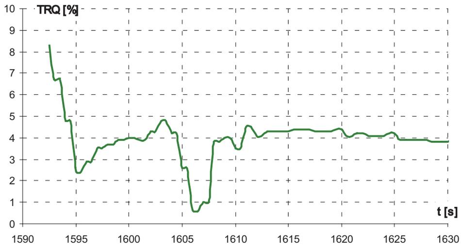
Fig. 20. Variations of the engine torque during the second restart
