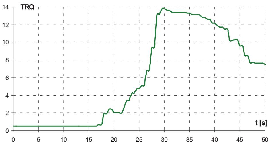
Fig. 6. Variations of the engine torque as a function of time during the engine start-up
