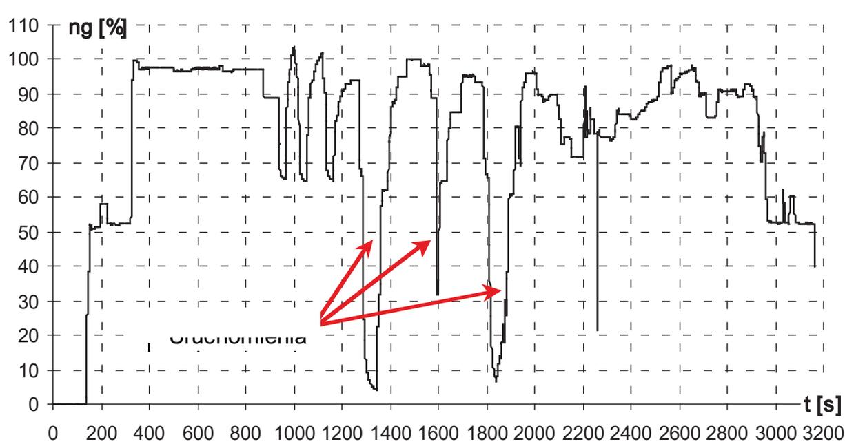
Fig. 13. Variations of the engine rpm during a test flight to check the functionality of restart in air
