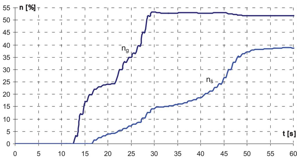
Fig. 3. Characteristic curves that depict rpm changes for the turbine generator and the airscrew during the start-up process as the function of time
