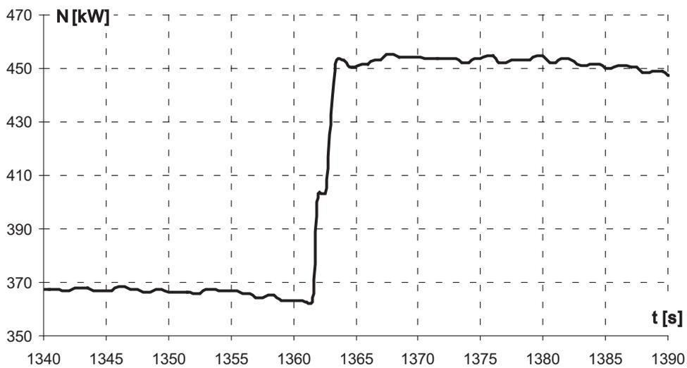
Fig. 22. Variations of the engine power during the first restart
