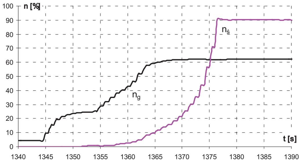
Fig. 16. Variations of the engine and airscrew rpm during the first restart
