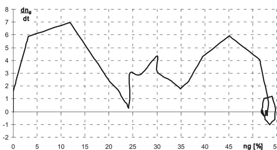
Fig. 12. Phase diagram for variations of the turbine generator rpm during the engine start-up
