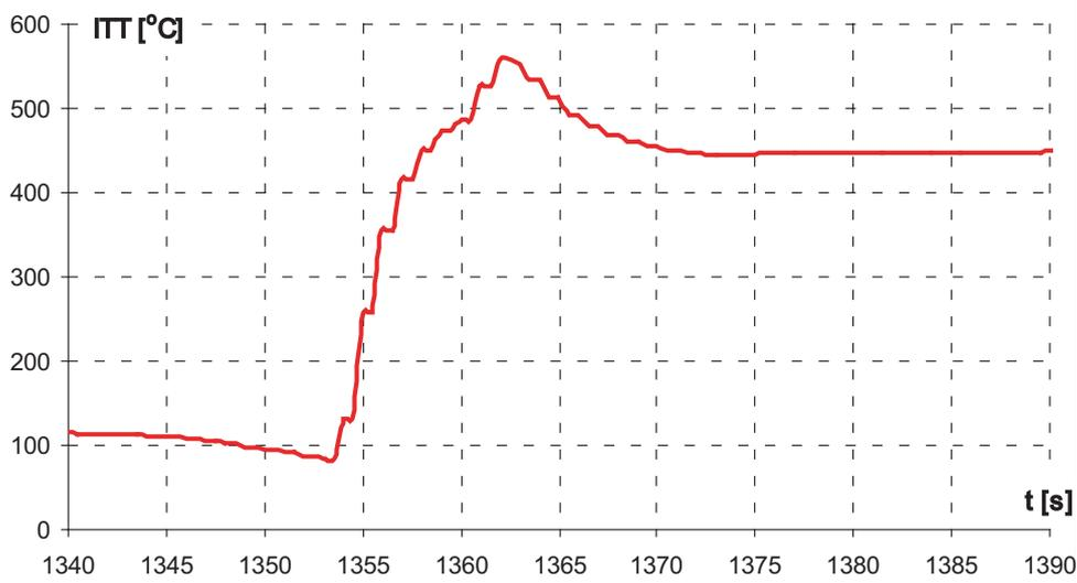
Fig. 23. Variations of exhaust gas temperature in between the turbines during the first restart
