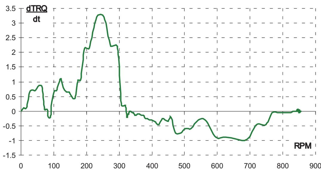
Fig. 9. Dynamics (acceleration) of the engine torque as the function of the airscrew rpm during the start-up process
