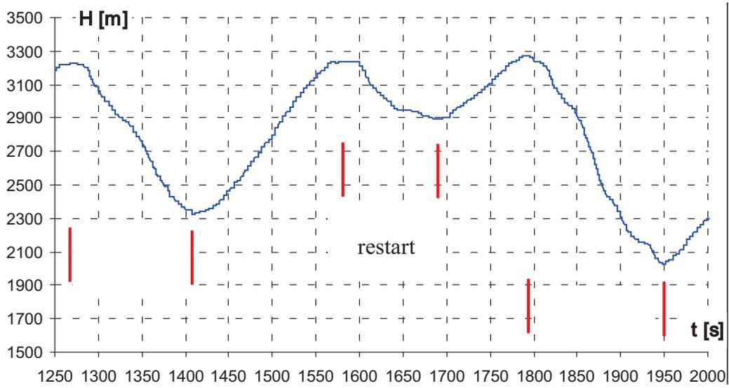
Fig. 14. Variations of the flight altitude associated with engine restart in air
