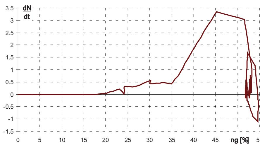
Fig. 11. Dynamic variations of the engine power as a function of the turbine generator rpm during the engine start-up
