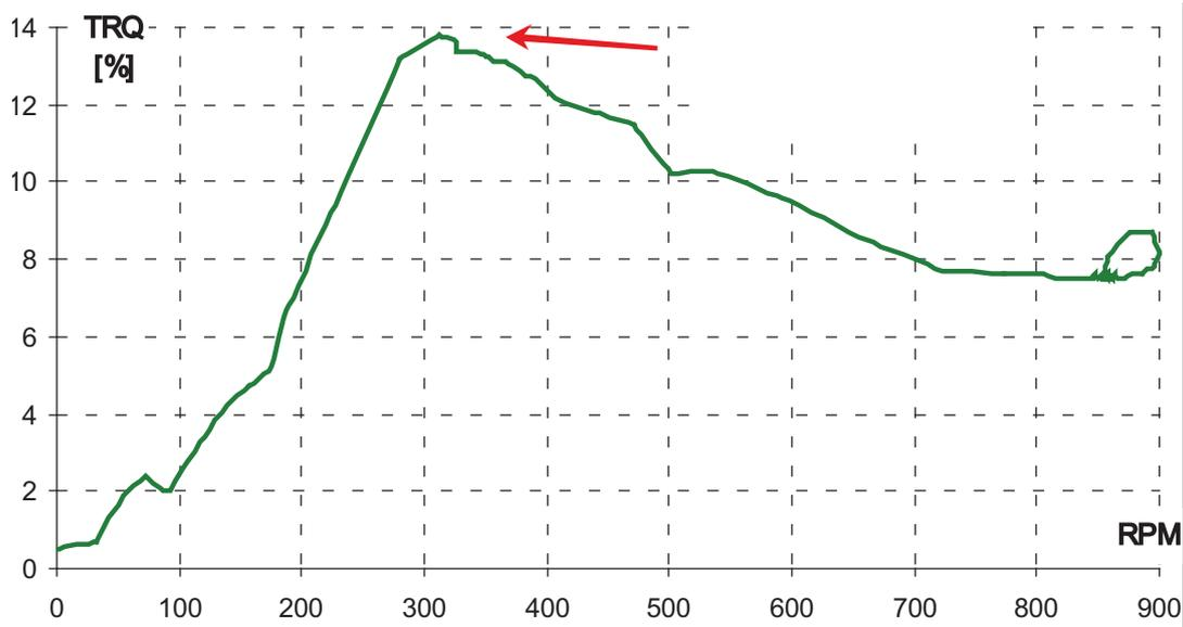
Fig. 8. Variations of the torque as a function of the airscrew rpm
