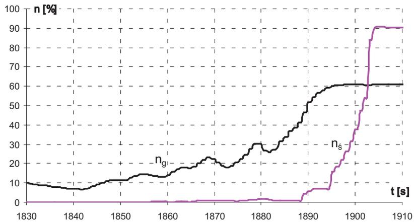
Fig. 18. Course of changes in engine speed and propeller during start of the third (emergency)
