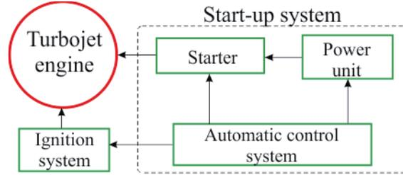
Fig. 1. Schematic diagram of the start-up system [3]
