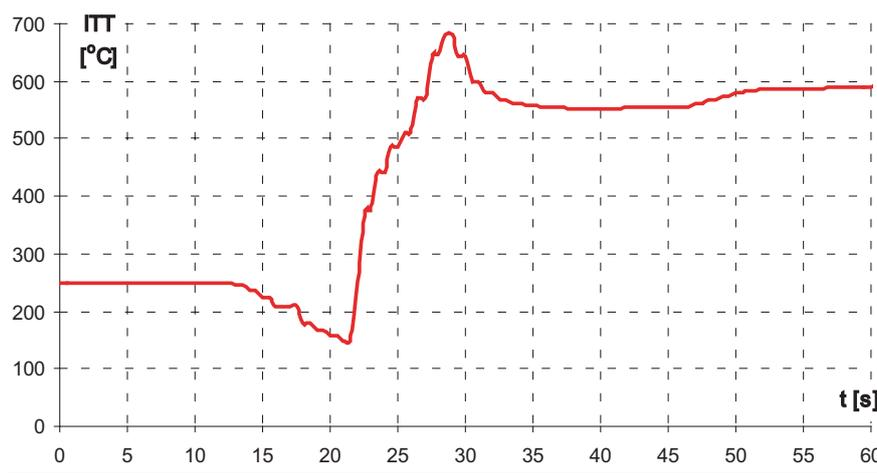
Fig. 10. Temperature variations in the area in between the turbines during the engine start-up
