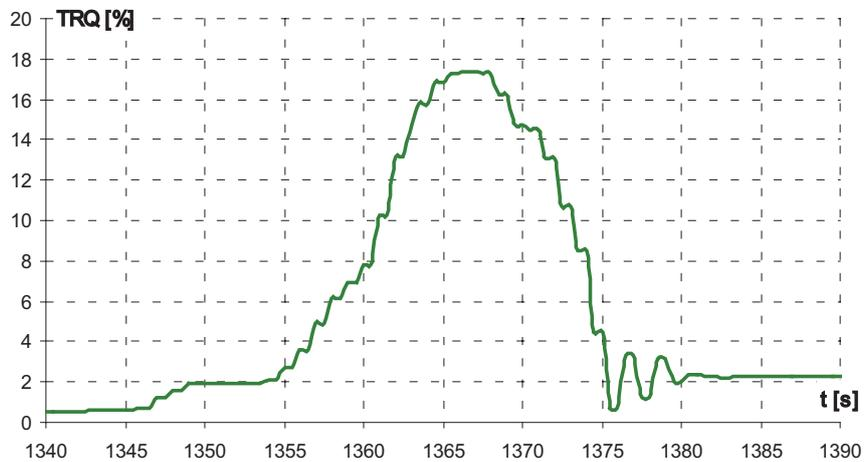
Fig. 19. Variations of the engine torque during the first restart
