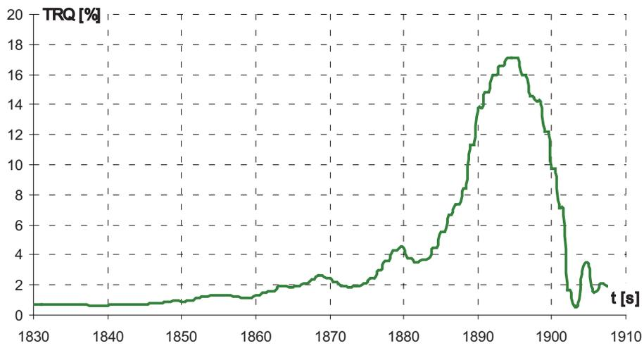
Fig. 21. Variations of the engine torque during the third restart
