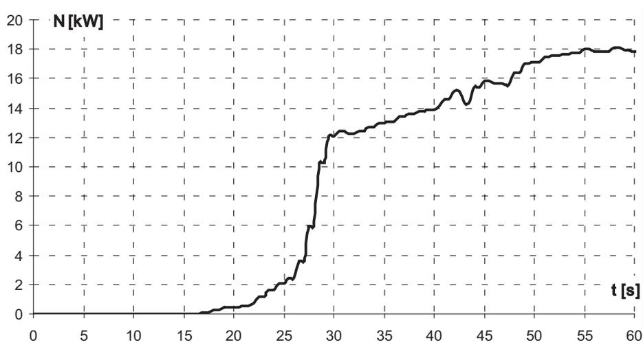
Fig. 7. Curve for power variations of the driving unit during start-up of the - PT6A-25C engine
