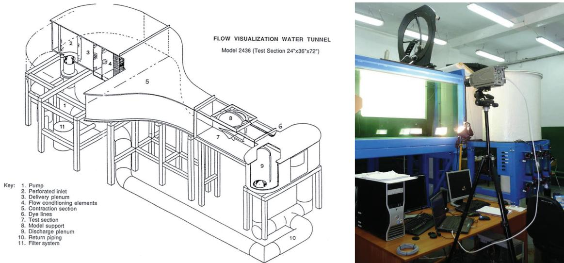
Fig. 1 Rolling Hills Research Water Tunnel Model 2436 [7]
