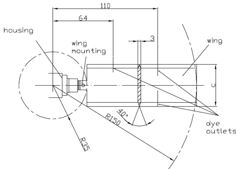
Fig. 4. Wing geometry
