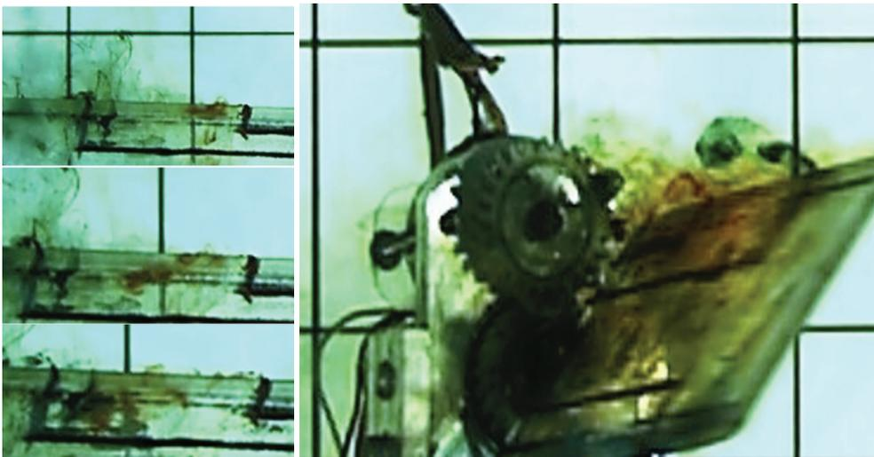
Fig. 6. Spanwise flow of LEV
