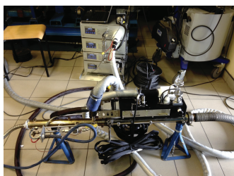
Fig. 4. The view of the analyser for on-road emission testing of vehicles: a) Ecostar by Sensors, b) M.O.V.E by AVL
