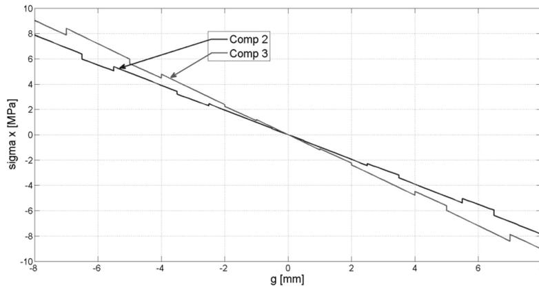
Fig. 14. Comparison of stress distribution of modified polymer-wood composites with soft and hard outside layers
