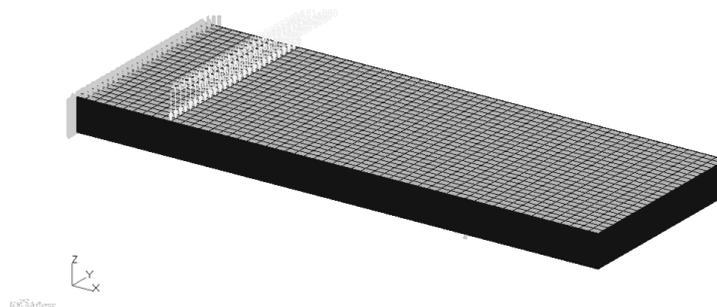
Fig. 2. FEM model of the polymer-wood composite
