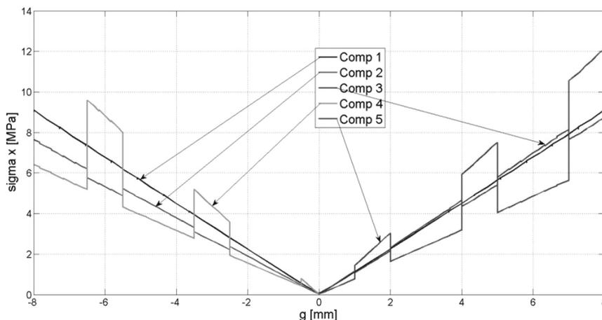
Fig. 12. Von Misses stresses for all types of analysed composites
