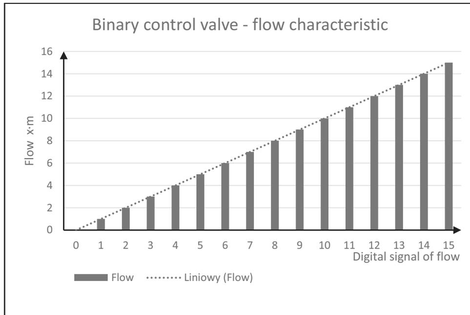
Fig. 3. Characteristics of flow through binary multi-valve
