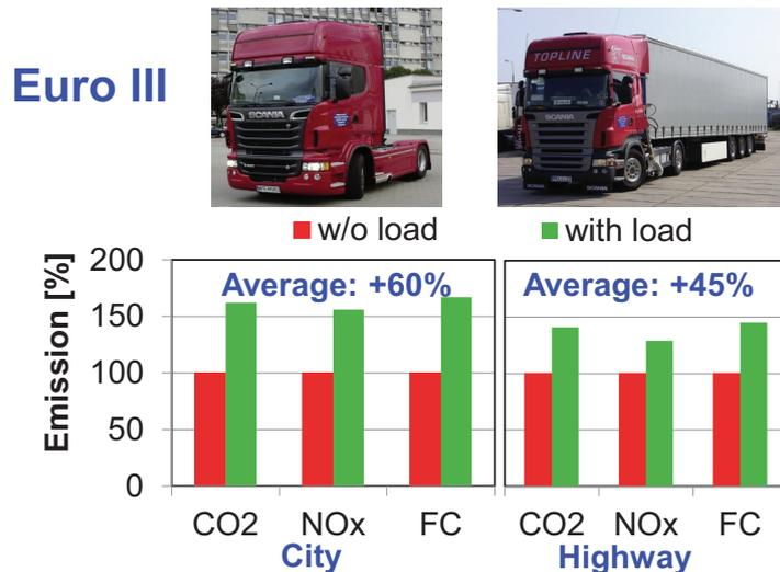
Fig. 14. Exhaust emissions test results for heavy-duty vehicles
