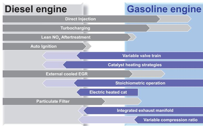
Fig. 5. Technology transfer between Diesel and Gasoline engines [5]
