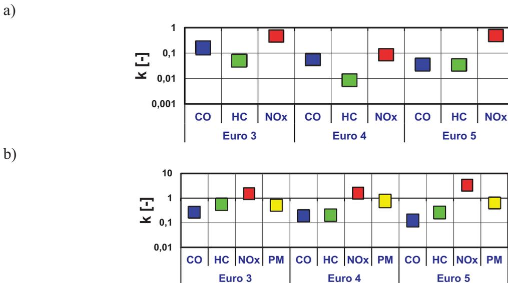
Fig. 12. Comparison of the vehicle exhausts emissions using different vehicle emission categories: a) gasoline engine, b) diesel engine
