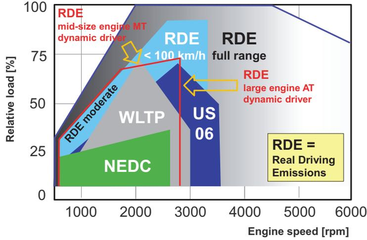
Fig. 10. Engine operating parameters in various emissions tests [16]
