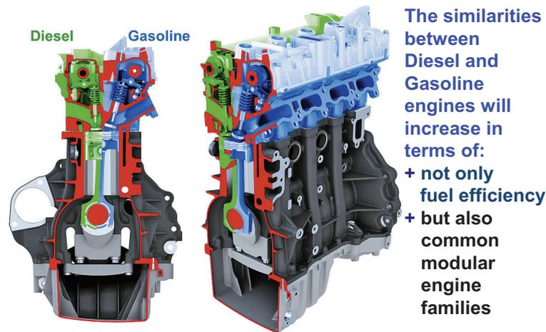
Fig. 6. AVL – Modular Diesel / Gasoline engine concept [6]
