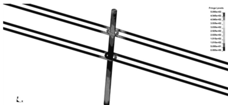
Fig. 8. Coupler deformation and tensions
