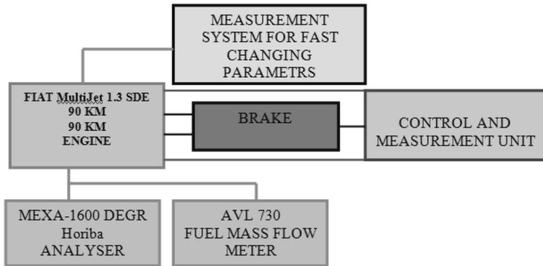
Fig. 1. Block diagram of the research stand
