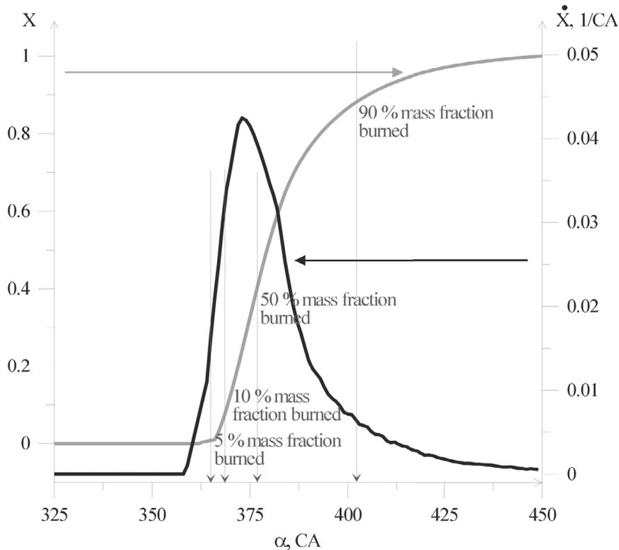
Fig. 2. Example characteristic curves of the relative quantity and rate of heat release during the process of combustion in the FIAT engine running following the load characteristics
