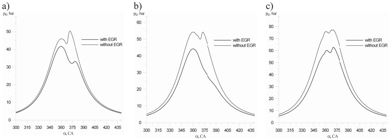
Fig. 4. The open indicator diagrams of the engine with and without the exhaust gas recirculation system, respectively, running according to the load characteristics at: a)  $n=1200$  rpm and under a load of  $M_o=20$  Nm; b)  $n=1750$  rpm and under a load of  $M_o=20$  Nm; c)  $n=3000$  rpm and under a load of  $M_o=20$  Nm
