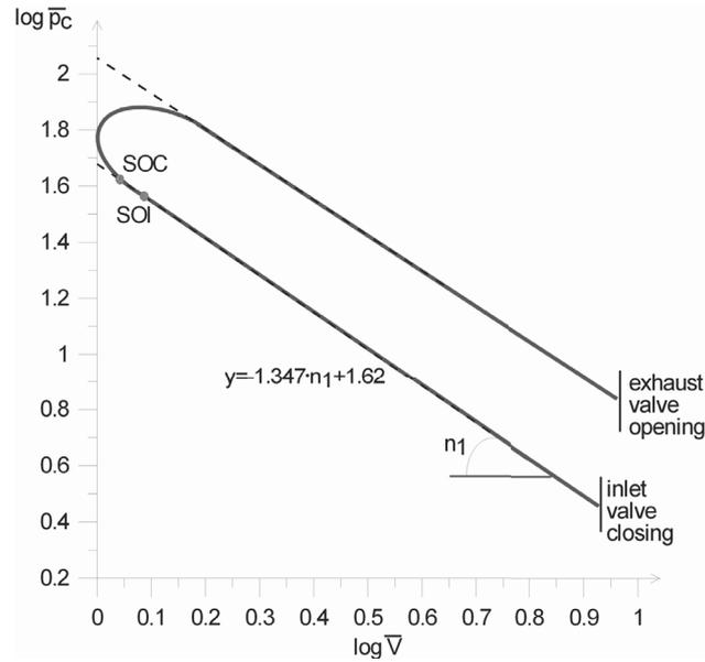
Fig. 3. The double logarithmic scale indicator diagram for the engine running following the load characteristics at  $n=1200$  rpm and under a load of  $M_o=80$  Nm, where: SOI – fuel injection process start, SOC – combustion process start
