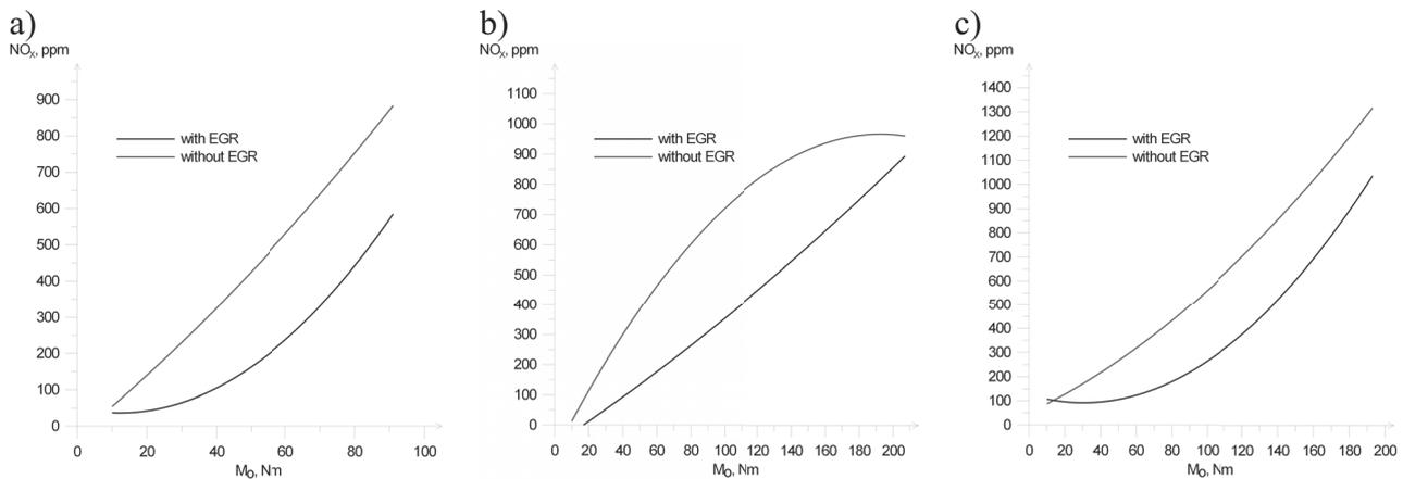
Fig. 6. Nitrogen oxide concentrations for the engine, respectively, with and without the exhaust gas recirculation system running according to the load characteristics at  $n=1200$  rpm, 1750 rpm and 3000 rpm
