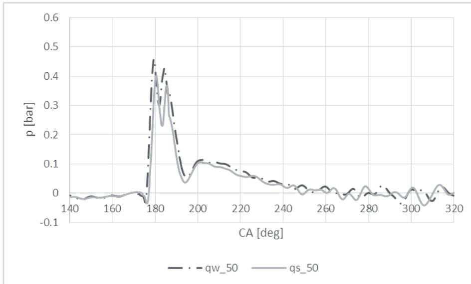
Fig. 4. Comparison of the net heat release rate  $q$  for the nominal state ( $qw_{50}$ ) and the state of clogged injector nozzles ( $qs_{50}$ ) for specific loads 50 kW
