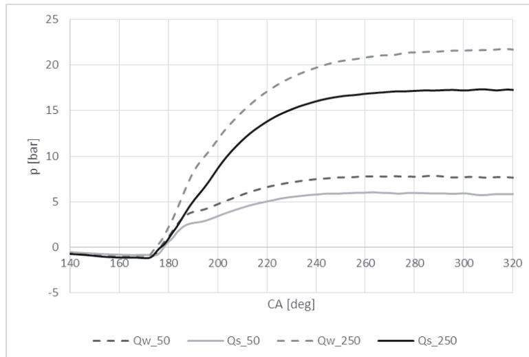
Fig. 3. Comparison of the net generated heat  $Q$  for the nominal state ( $Qw50$ ;  $Qw250$ ) and the state of fuel pump leakage ( $Qs50$ ;  $Qs250$ ) for specific loads 50 and 250 kW
