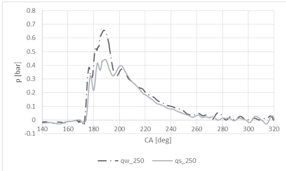
Fig. 5. Comparison of the net heat release rate  $q$  for the nominal state ( $q_{w250}$ ) and the state of clogged injector nozzles ( $q_{s250}$ ) for specific loads 250 kW
