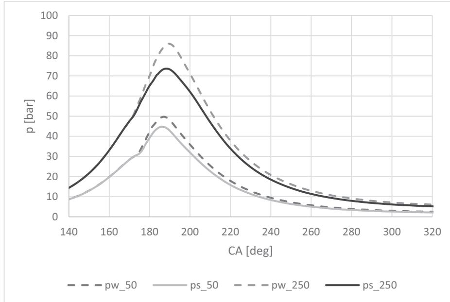
Fig. 1. Comparison of the indicator diagram for the reference state ( $p_{w50}$ ;  $p_{w250}$ ) and the simulation of fuel pump leakage ( $p_{s50}$ ;  $p_{s250}$ ) for engine power 50 kW and 250 kW
