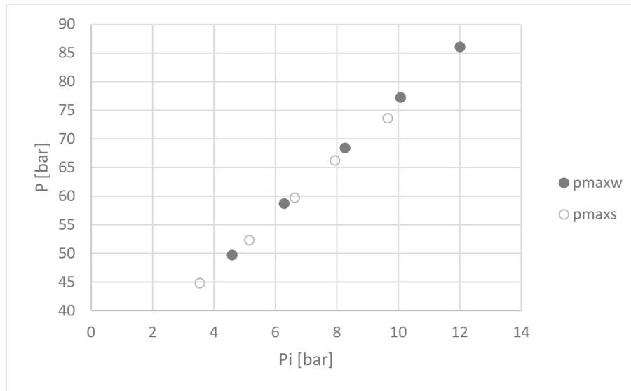
Fig. 2. Comparison of the maximum pressure in the cylinder as a function of mean indicated pressure  $p_i$ :  $p_{maxs}$  – simulation,  $p_{maxw}$  – reference state
