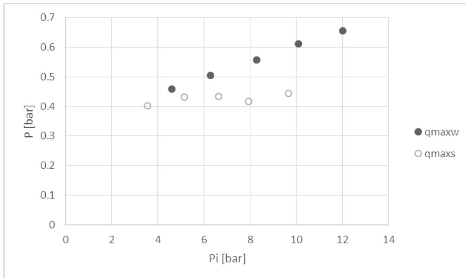
Fig. 6. Comparison of the max of net heat release rate  $q$  as a function of mean indicated pressure  $p_i$ :  $q_{maxs}$  – simulation,  $q_{maxw}$  – reference state
