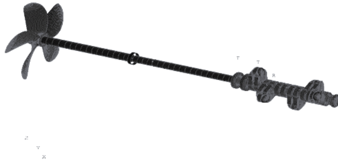
Fig. 1. FEM model of a typical marine propulsion system
