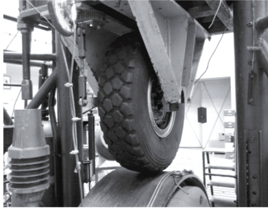
Fig. 5. Mlot 3T test stand with brake and wheel mounted during tests (source: ILOT)
