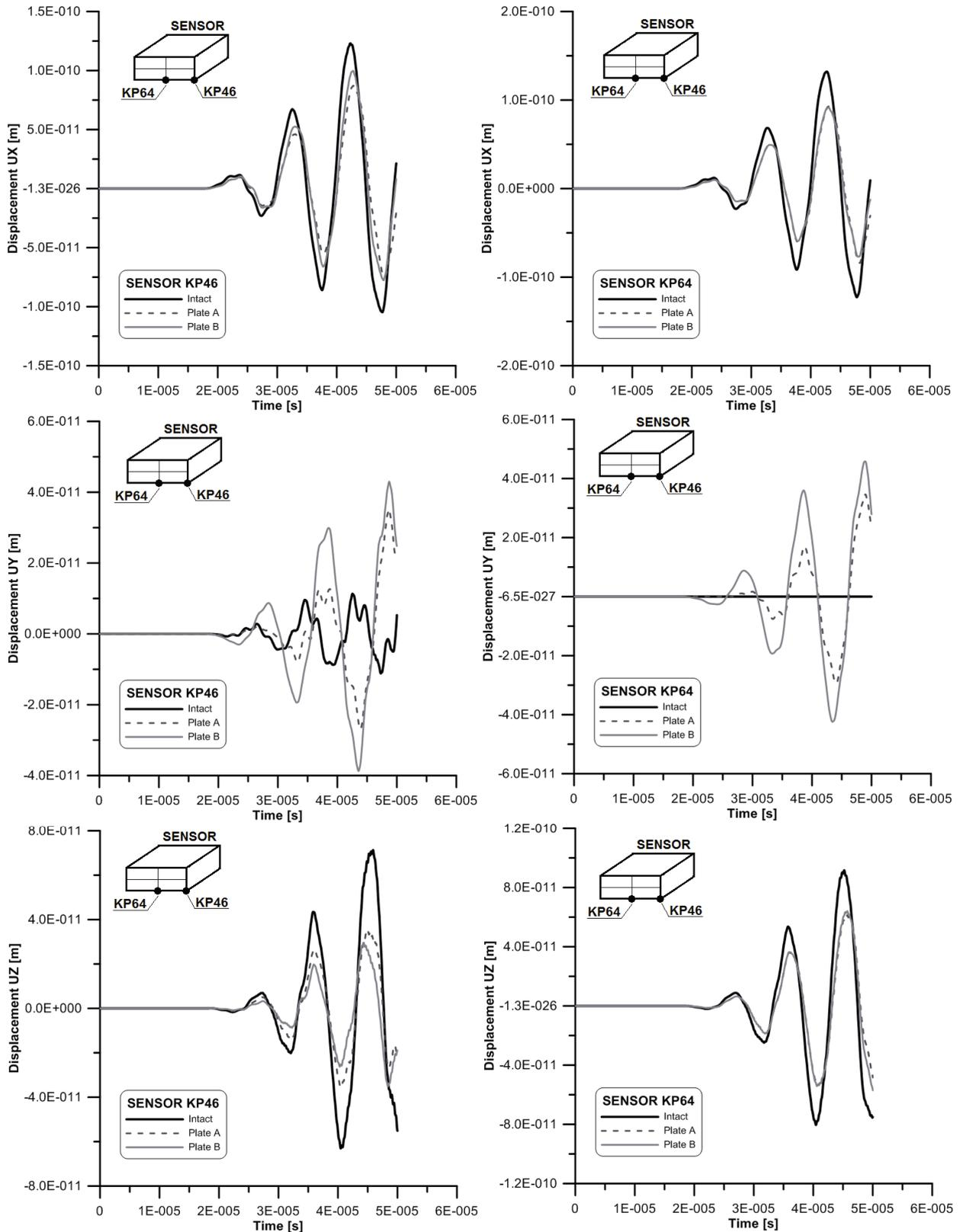
Fig. 6. The component of the displacement versus time obtained for the plate a, plate B and the intact structure
