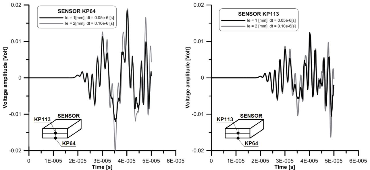
Fig. 5. The voltage amplitude versus time for two different element size and time step
