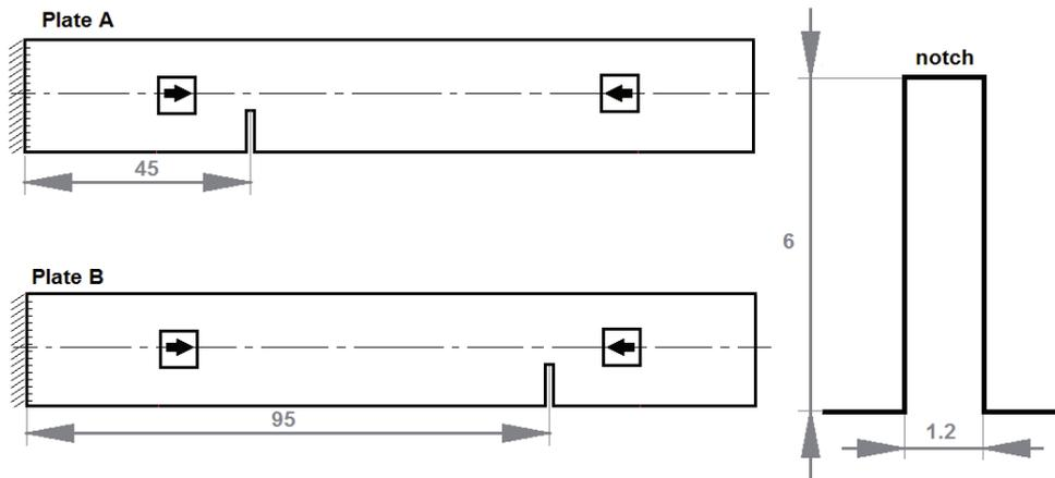
Fig. 2. The assumed localization of the notch in the structure A and B
