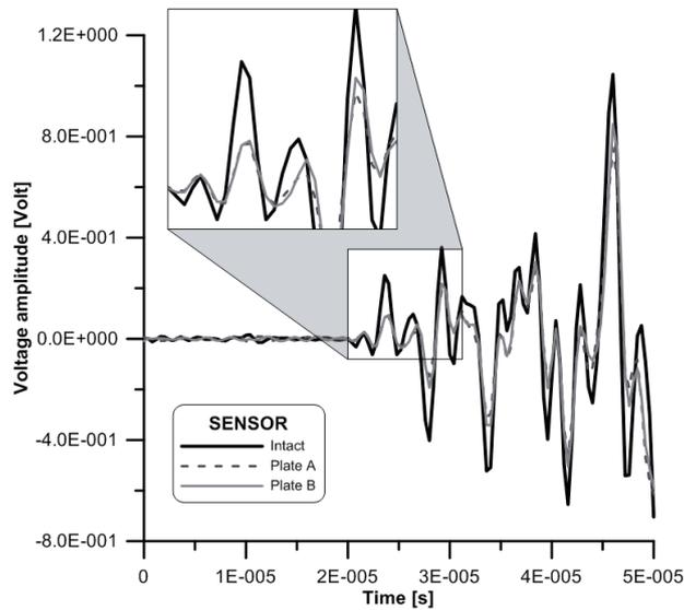
Fig. 8. The voltage amplitude versus time obtained for the plate A, B and the intact structure (experimental findings)
