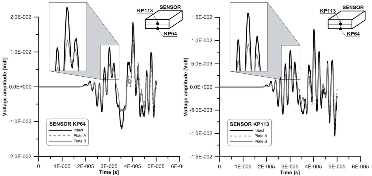
Fig. 7. The voltage amplitude versus time obtained for the plate A, B and the intact structure
