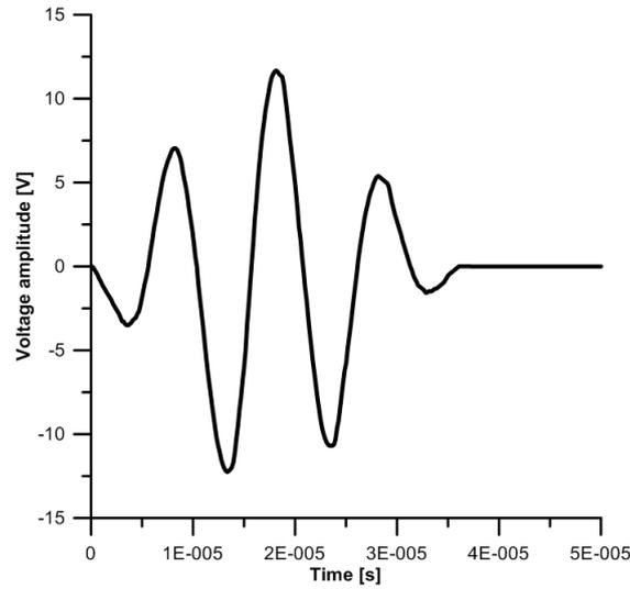
Fig. 3. The real tone burst excitation signal
